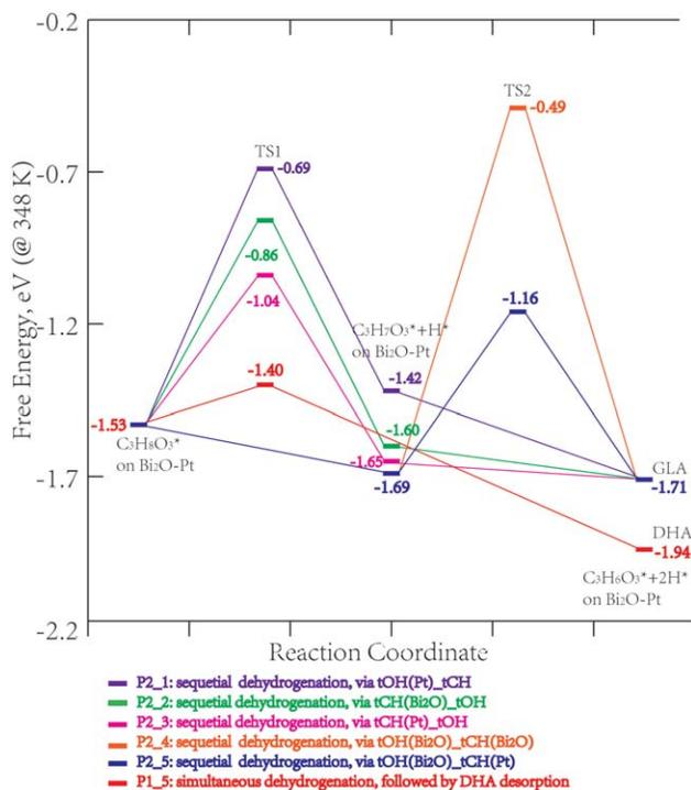
**Figure 8. Energy diagram for primary vs. secondary hydroxyl oxidation of glycerol on the Pt-Bi surface.**
