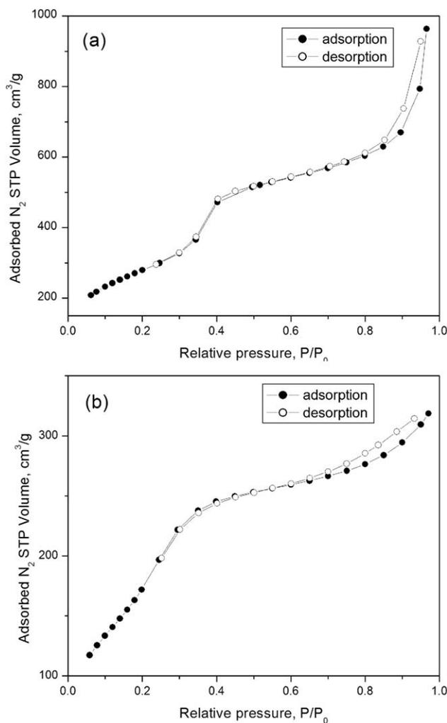
**Figure 2. Adsorption and desorption isotherms for (a) MCM-41 and (b) Bi-MCM-41.**
