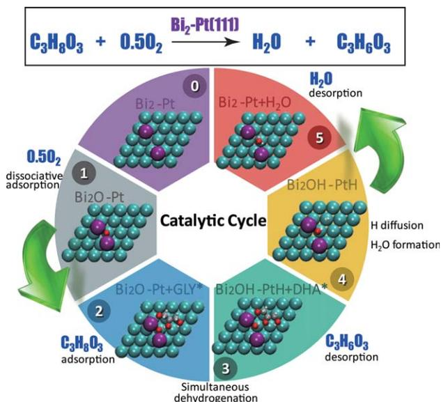
**Figure 9. Proposed catalytic cycle of Pt-Bi for DHA ( $C_3H_6O_3$ ) formation from glycerol ( $C_3H_8O_3$ ).**
