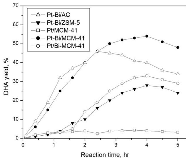
**Figure 4. Kinetic behavior of different catalysts for glycerol conversion to DHA.**
