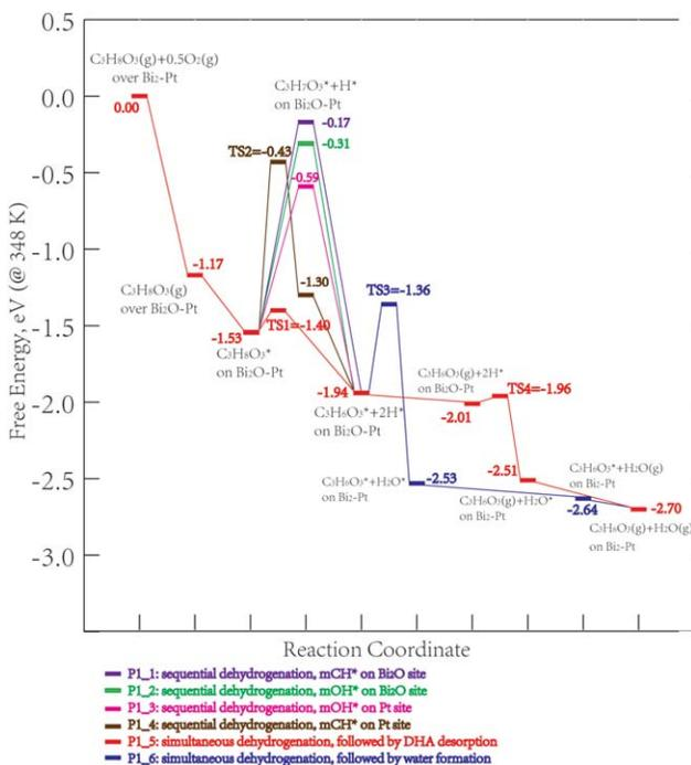
**Figure 7. Energy diagram for DHA formation pathways on the Pt-Bi surface.**
