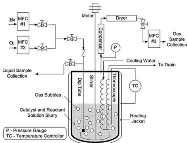
**Figure 1. Pressure semi-batch reactor system.**
