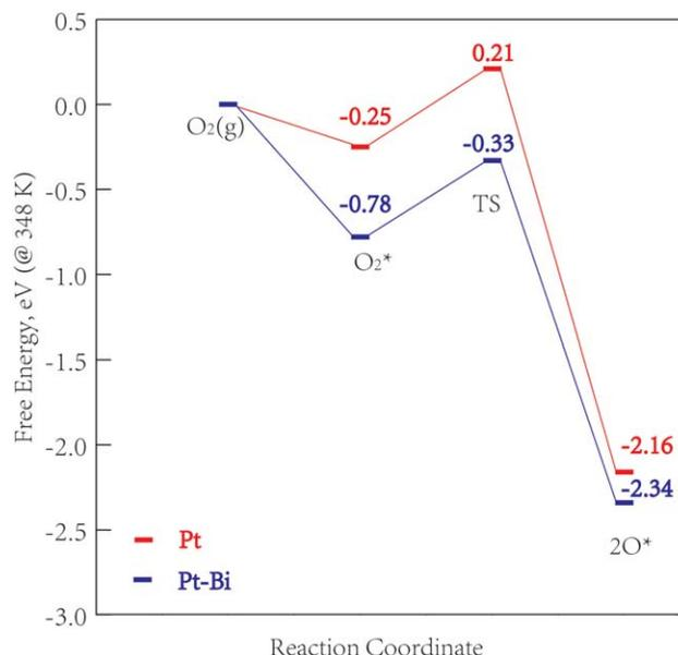
**Figure 5. Energy diagram for dissociative adsorption of oxygen on Pt and Pt-Bi surfaces.**
