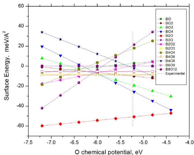
**Figure 6. Phase diagram for oxidized bismuth models on Pt(111) surface.**
