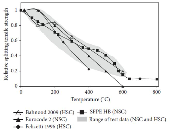
**Figure 4 :** Variation in relative splitting tensile strength of concrete as a function of temperature.
