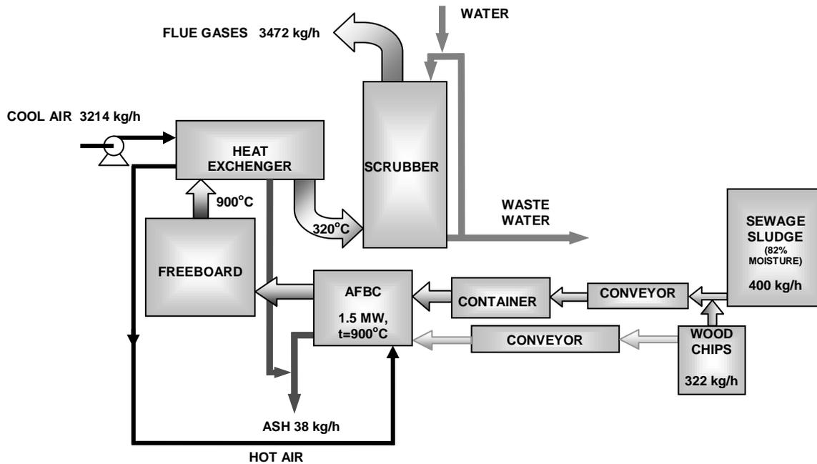
Fig. 1. A scheme of the proposed technology for the incineration of wet sewage sludge
