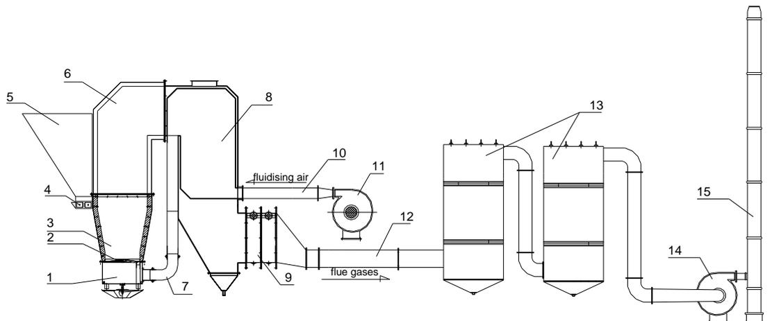
Fig. 2. A scheme of the installation for burning sewage sludge built at the Waste Water Treatment Plant at Niepołomice
