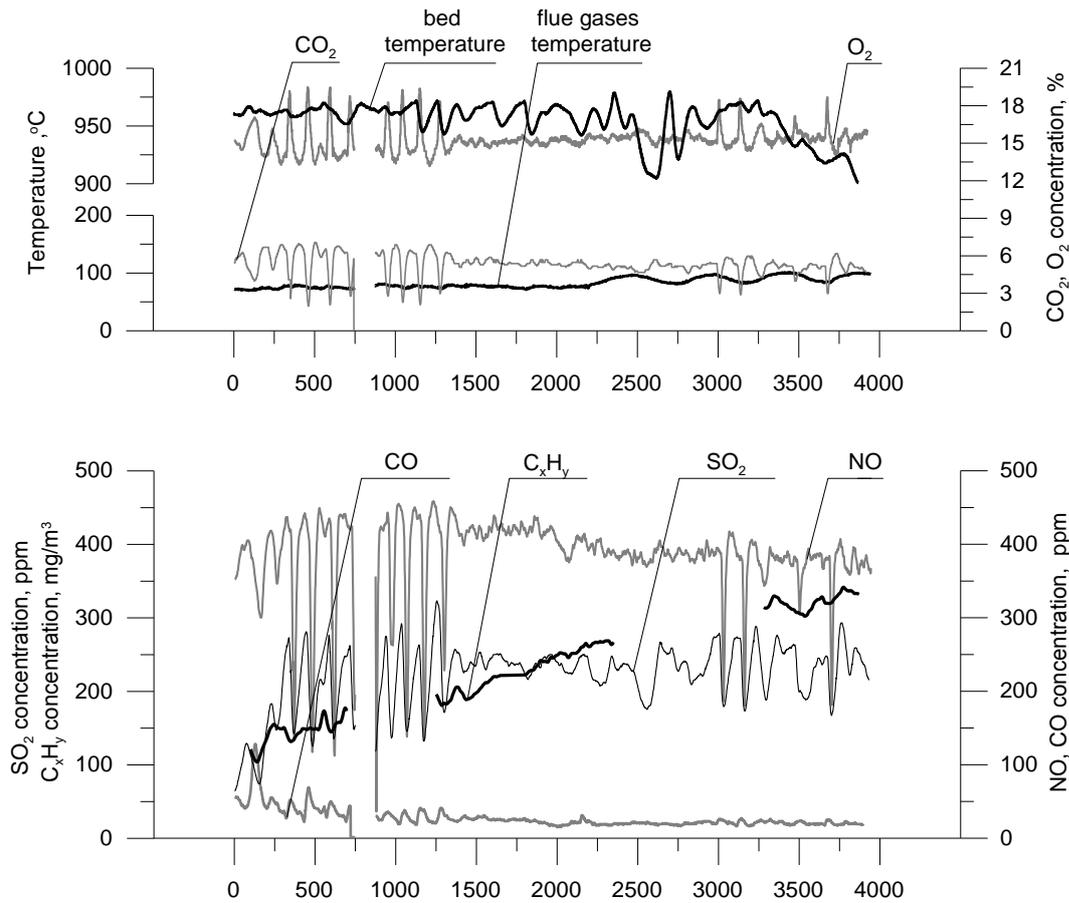
Fig. 3. Temperature records and flue gas concentrations observed when sewage sludge was burned in the 1.5 MW fluidised bed combustor
