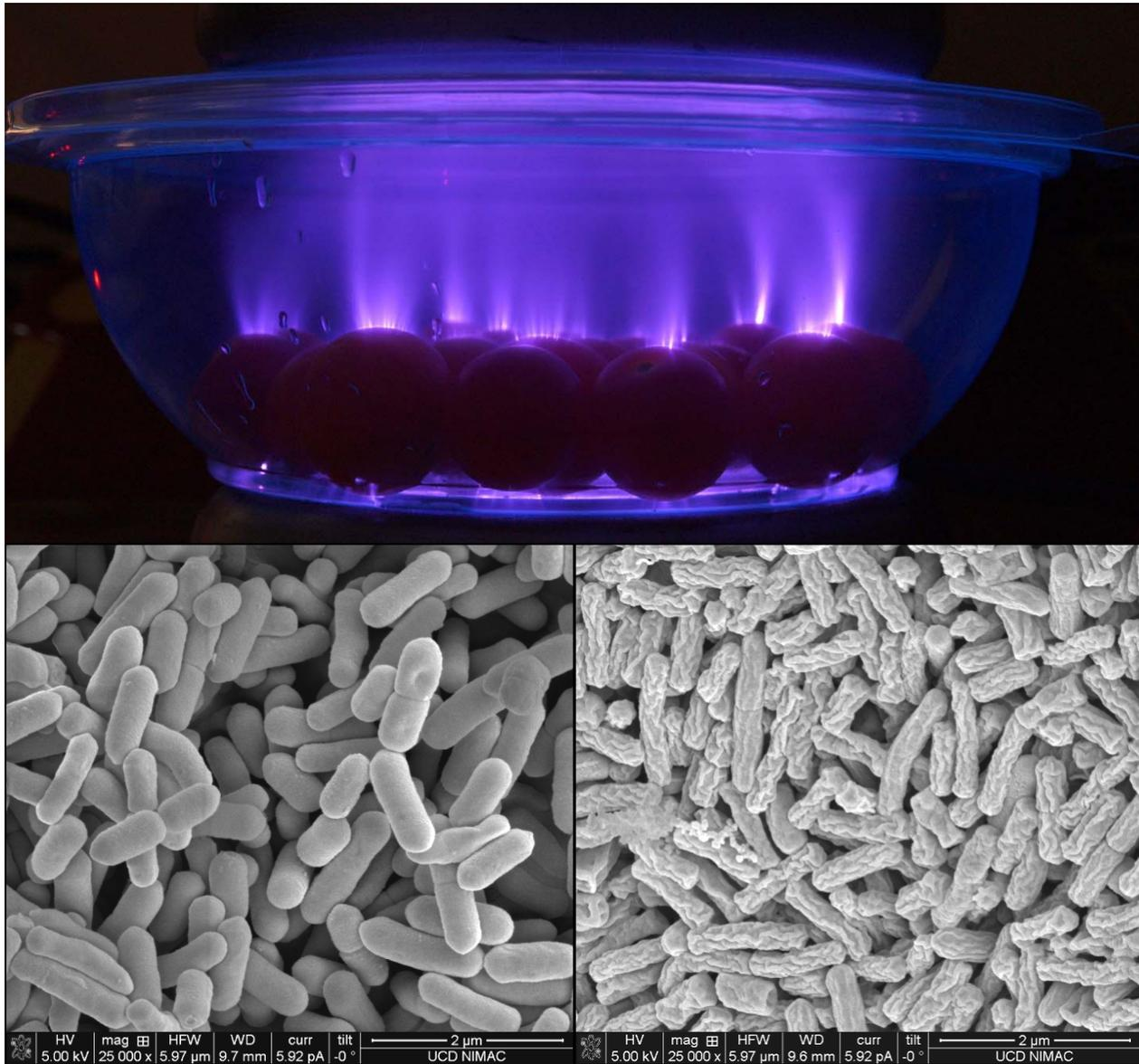
Fig. 1. Top: DBD plasma treatment of tomatoes in-package, a high-voltage electrode (60 kV RMS). Bottom: Scanning electron micrographs of untreated and plasma treated *L. monocytogenes* NCTC 11994.
