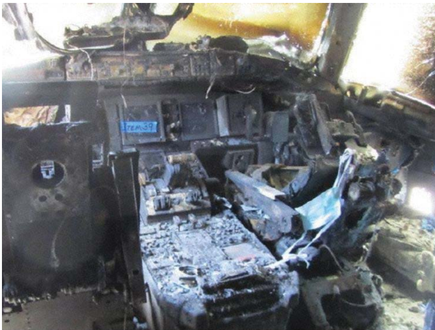
Figure 1. Electrical fire destroyed cockpit of EgyptAir 667
