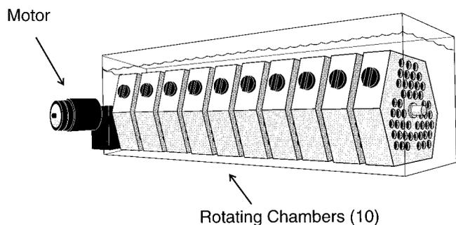
Fig. 1. Diagram of the suspended solids testing apparatus (SSTA) showing motor and rotating chambers in tank.
