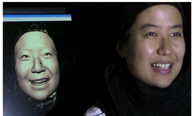
Fig. 5 Geometric video acquired at 60 fps with our system. The left figure is the real-time reconstructed 3-D result. The right figure is the subject.
