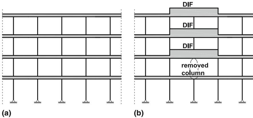
**Fig. 1** Frame loading scheme: **a** intact frame, **b** column loss at second floor
