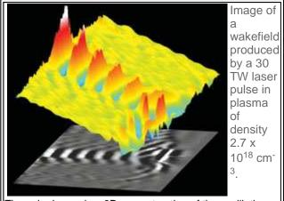
The color image is a 3D reconstruction of the oscillations, and the grey scale is a 2D projection of the same data. These waves show curved wave-fronts, an important feature for generating and accelerating electrons that had been predicted, but never before seen.
