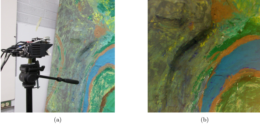
Figure 3: Data Set Acquisition. (a) Texel camera and landscape. (b) Example EO image captured using the texel camera.
