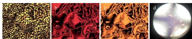
Fig. 5 POM textures of compound 4 in the homeotropic aligned cell (a) at 178 °C, (b) at 175 °C, and (c) at 65 °C. (d) Conoscopic pattern of compound 4 in the nematic phase in homeotropic dark state at 173 °C.
