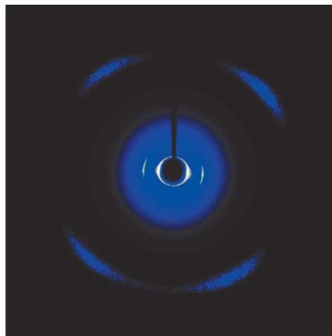
**Fig. 5** X-Ray diffraction pattern of a single domain  $B_2$  phase of **4e**. The angle between the directions of the small and large angle reflections yields the molecular tilt angle to be  $37 \pm 2^\circ$ .
