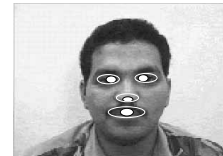
Fig. 4. Fourbull's-Eyes template used to subjectively test FFL algorithm's accuracy.
