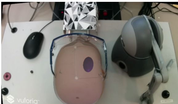
Fig. 6 Each virtual ellipsoid is a target with random 3D position, size, and orientation in 3D, used to provide a well-posed targeting task
