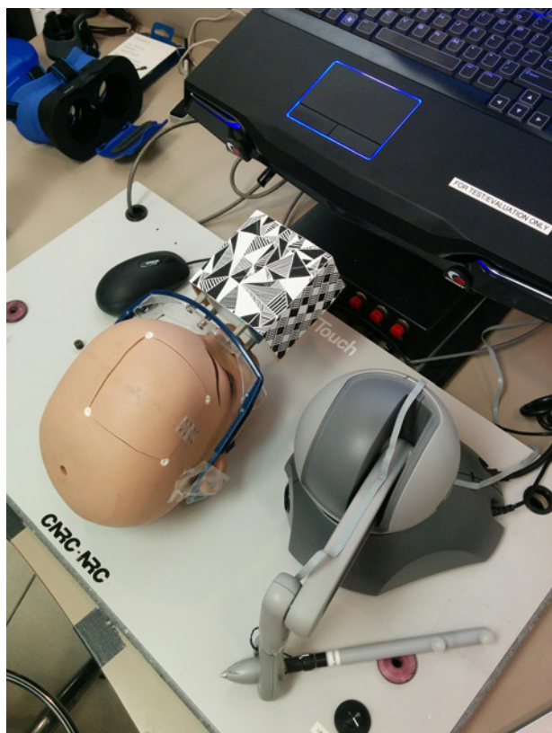
Fig. 3 NeuroTouch haptic interface, mannequin head, and Vuforia image tracking cube. These are the physical input devices
