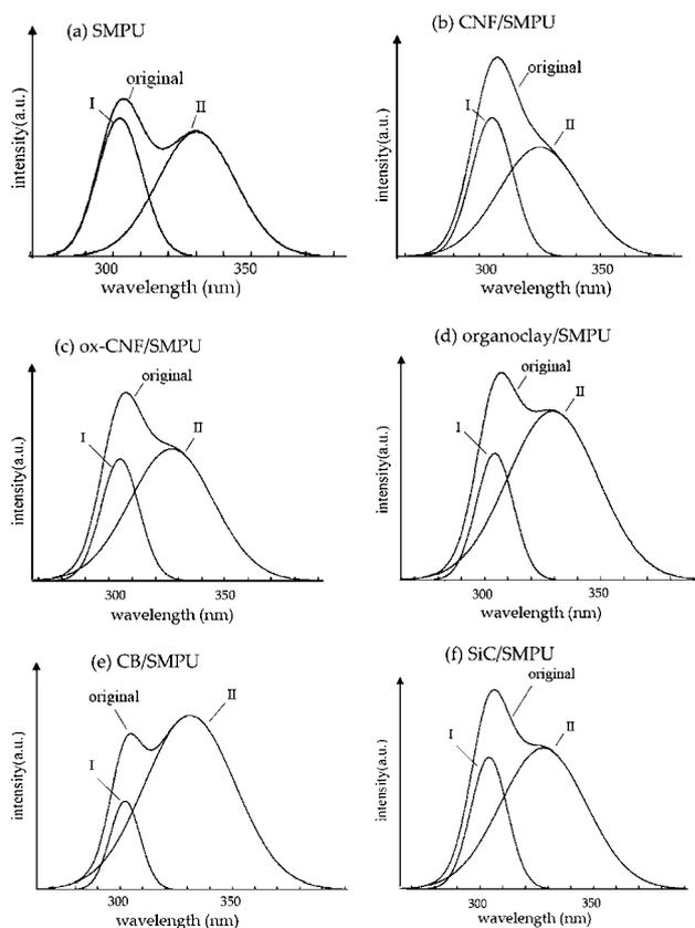
**Fig. 4** Fluorescence emission spectra of SMPU composites taken at room temperature. (a) pristine SMPU, (b) CNF–SMPU, (c) ox-CNF–SMPU, (d) organoclay–SMPU, (e) CB–SMPU and (f) SiC–SMPU. Note the significant reduction in the intensity of peak I in composites of ox-CNF, CB, and organoclay. Peak I was located at around 305 nm, whereas peak II was located at around 330 nm. Each composite contained 1 wt% filler.
