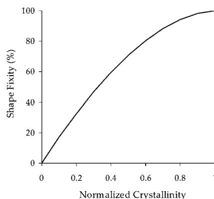
**Fig. 9** The predictions of eqn (6) for the relationship between SF and the extent of soft segment crystallinity. Predicted curve was calculated using arbitrary values, although the overall trend of the predicted curve does not change significantly with selection of parameters.
