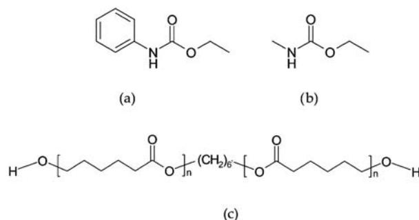
**Fig. 1** Chemical structures of (a) phenyl urethane, (b) *N*-methyl urethane, (c) poly(caprolactone)diol ( $M_w = 4000$  g mol<sup>-1</sup>).
