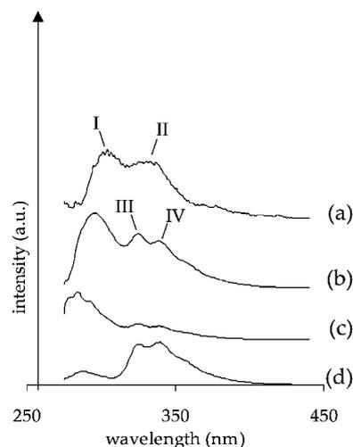
**Fig. 3** Fluorescence emission spectra of compounds. Curve (a) solid SMPU, curve (b) dilute SMPU solution in DCM, curve (c) dilute *N*-methyl urethane solution in DCM and curve (d) dilute phenyl urethane solution in DCM. All spectra were taken at room temperature. The concentration of dilute solutions was about 1 g L<sup>-1</sup>.
