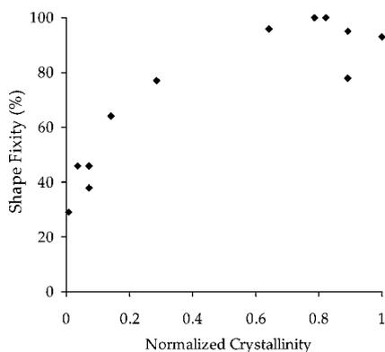
**Fig. 8** The experimental data on the relationship between SF and the extent of soft segment crystallinity of SMPU composites filled with organoclay, CNF, ox-CNF, SiC, and CB. Experimental data (filled squares) were taken from previous reports.<sup>4,12</sup> Normalized soft segment crystallinity values were determined by dividing the value of soft segment crystallinity of the specific composite by that of the pristine SMPU.
