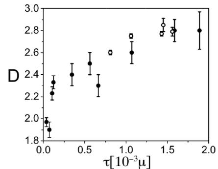
FIG. 4. Fractal dimension  $D$  of dislocation cell structures for single crystals deformed at different stresses. Full circles: fractal dimension from phase-field simulations. Open circles: fractal dimension of [100]-oriented Cu single crystals [7].
