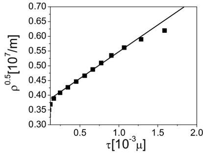
FIG. 2. Evolution of the square root of the dislocation density with the applied shear stress with a fitted relation  $\tau \sim \mu b \sqrt{\rho}$ .
