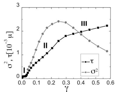
FIG. 1. Calculated strain-stress curve and the evolution of the variance of the dislocation density, as described in the text. The stress is given in units of  $10^{-3} \mu$ .
