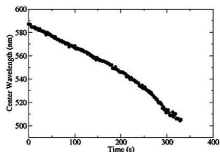
**Fig. 3** Change in the central reflection wavelength of the N\* phase of compound **2** at 75 °C using continuous UV irradiation ( $\lambda_{\text{max}} = 365 \text{ nm}$ ,  $5.0 \text{ mW cm}^{-2}$ ).
