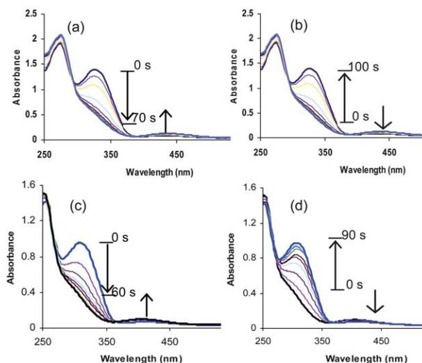
**Fig. 1** Photoisomerization of compounds **1** and **2** monitored by UV-Vis spectroscopy: *trans* to *cis* isomerisation by 365 nm irradiation of **1** (a) and **2** (c) and reversible *cis* to *trans* isomerisation by 440 nm irradiation for **1** (b) and **2** (d).
