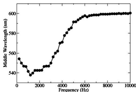
**Fig. 5** Peak reflections as a function of frequency under a 40 V electric field applied to the cell.
