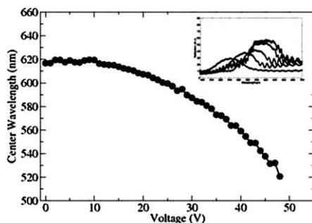
**Fig. 4** Center of the reflection wavelength vs. voltage in the N\* phase of compound **2** at 65 °C. Higher the electrical field, higher is the layer tilt and consequently the blue shift. The inset shows the measured reflection spectra under different voltages.
