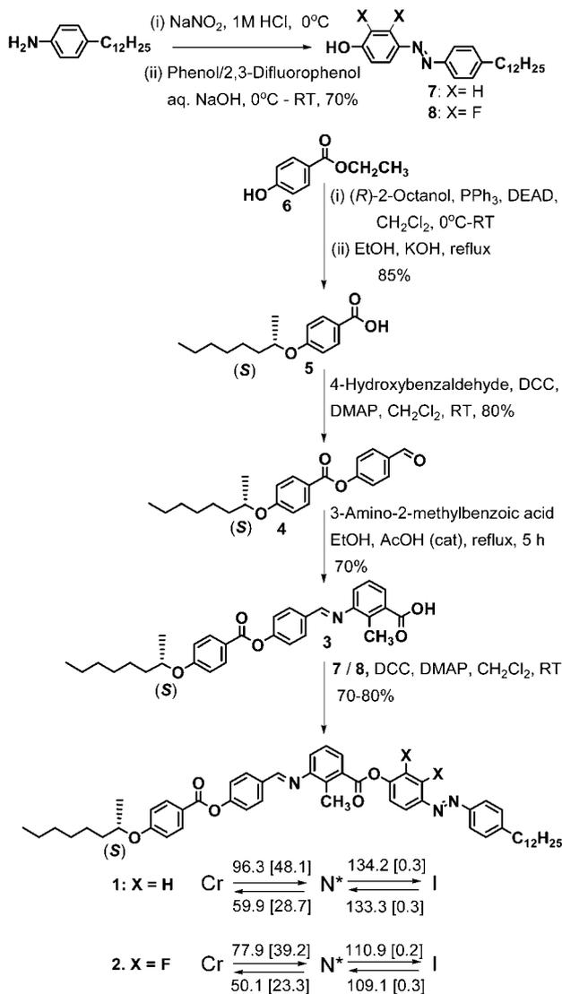
**Scheme 1** Synthesis, phase transition temperatures ( $T^\circ\text{C}$ ) and the corresponding enthalpies [ $\text{J g}^{-1}$ ] of the chiral banana-shaped molecules **1** and **2**. Abbreviations: Cr = crystal, N\* = chiral nematic, and I = isotropic.
