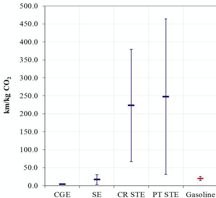
**Figure 6** Distance Traveled per kilogram of CO<sub>2</sub> Emitted
