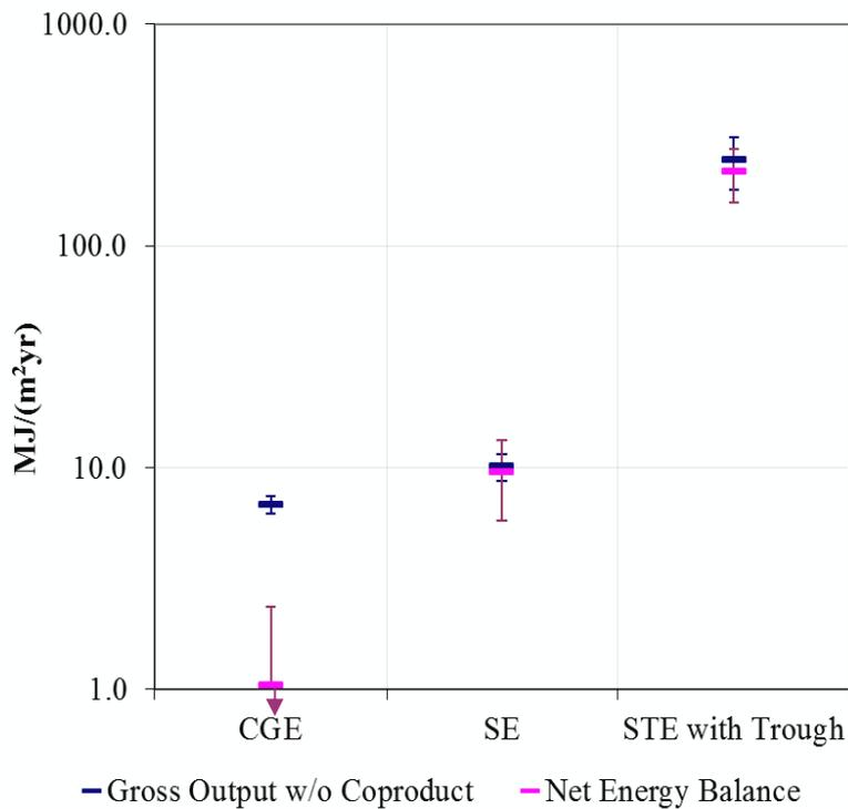
**Figure 1** Annual Energy Produced per Square Meter of Land Used for Corn Grain Ethanol (CGE), Switchgrass Ethanol (SE) and Solar Thermal Electric (STE)
