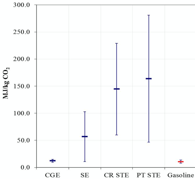
**Figure 3** Energy Produced (MJ) per kilogram of CO<sub>2</sub> Emitted. CR: Central Receiver, PT: Parabolic Trough.
