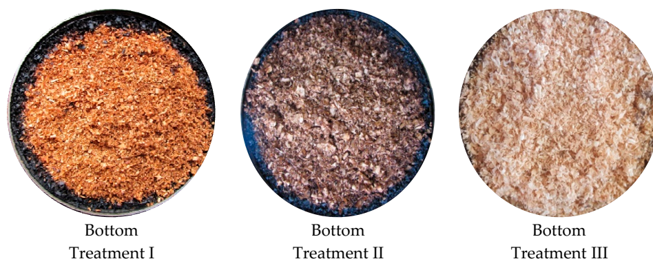
Figure 7. Top and bottom sections of the filter for three treatments: (I) wood shavings filter; (II) heat exchanger + wood shavings filter; and (III) oil bubbler + wood shavings filter.
