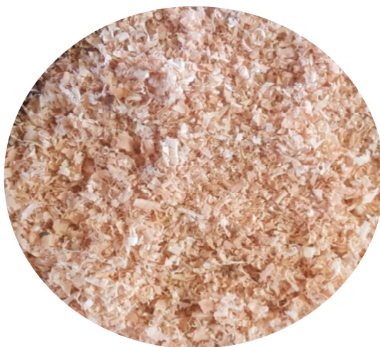
Figure 4. Wood shavings used as the filter medium for all treatments.
