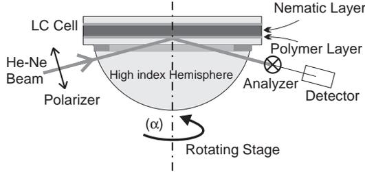
Fig. 2 – Setup for TIR study of the polymer layer and LC orientation near the glass surface via depolarization of the reflected He-Ne beam. The hemisphere and the bottom glass plate of the cell have the same high optical index ( $n_g = 1.802$ ) and we use index matching fluid to have a good contact between them.
