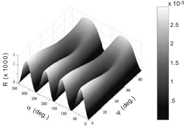
Fig. 4 – Simulation of the evolution of the TIR signal ( $R(\alpha)$ ) when the opening angle of fan distribution ( $\psi$ ) is increased. The plane of the fan is tilted by  $\theta = 26^\circ$  and  $\delta n_{\text{uniox}} = 0.04$ .
