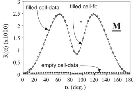
Fig. 3 – Experimental data and fit obtained on sample M (mechanical rubbing) filled and unfilled: (black dots) measurement on the empty cell; (gray dots) measurement on the filled cell; (gray line) fit of the filled cell with an isotropic AL and a homogeneous pretilted orientation of the LC having the nematic director along the rubbing direction. The fit allows us to determine  $n_{AL} = 1.734 \pm 0.002$ ,  $\beta = 4.7 \pm 0.2^\circ$  and  $\langle Q \rangle_{TIR} = Q_{bulk} \pm 0.1$ .
