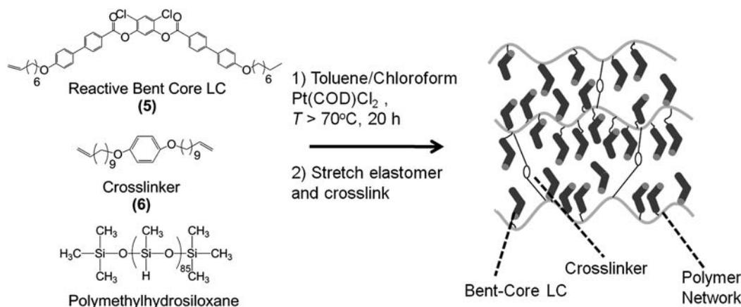
**Scheme 2** Synthesis of aligned bent-core liquid crystal elastomer (BCE).
