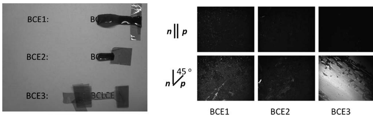
**Fig. 2** A photograph of the bent-core elastomers produced in this study (left) and polarizing optical micrographs of BCE 1–3 (right). BCE3 exhibits the best optical clarity. BCE4 is not shown but has optical quality comparable to BCE1 and BCE2. The polarizing optical microscopy frames show that BCE3 also has the highest birefringence, indicating better alignment of the LC side groups.
