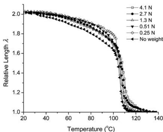
**Fig. 3** Thermoelastic behavior of sample BCE3 under different loads. The relative length  $\lambda$  is given by the ratio of the length of the sample at a given temperature to the sample length just above  $T_{NI}$ . A force of 0.25 N corresponds to a stress of 0.98 kPa.
