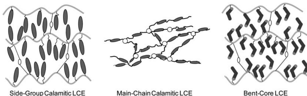
**Fig. 1** Schematic of different types of LCEs. Side-chain calamitic LCEs are made by attaching a rod-like mesogen as a side-group to a polymer network. Main-chain LCEs incorporate the mesogen into the backbone of the polymer network. Side-group bent-core LCEs (BCEs) have bent-core mesogenic side groups attached to the polymer network *via* a flexible spacer.
