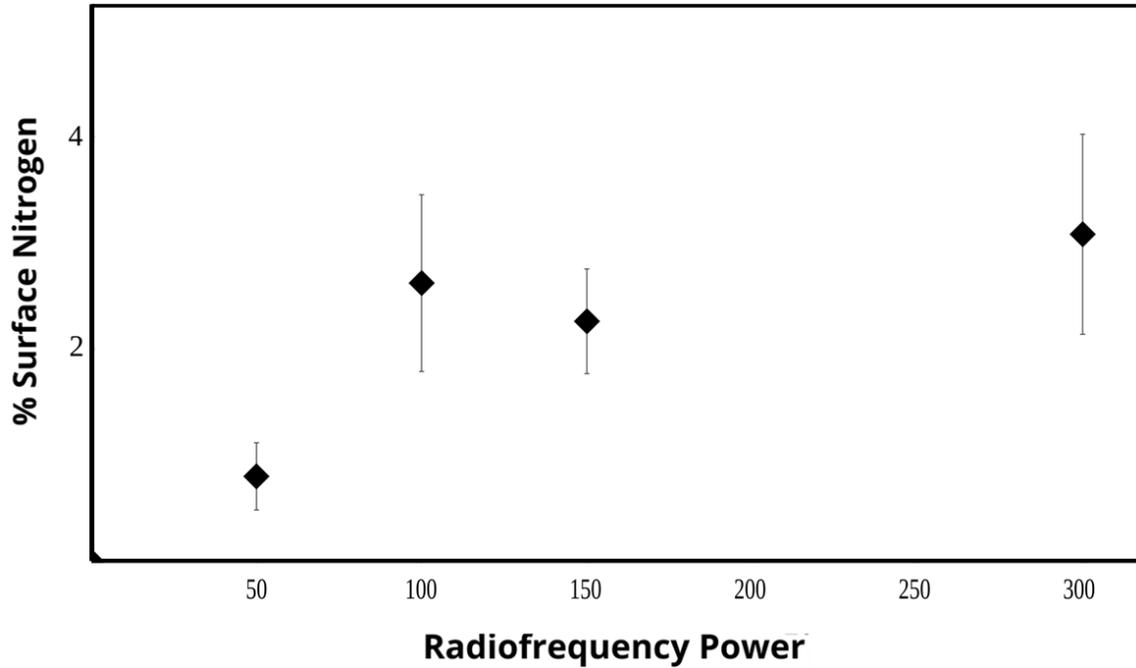
**Figure 3:** Surface nitrogen content on PVA treated with O<sub>2</sub> plasma as a function of RF power. Values approached steady state at values higher than 100 W according to a one-way ANOVA with equal variances (N = 5, p < 0.05).
