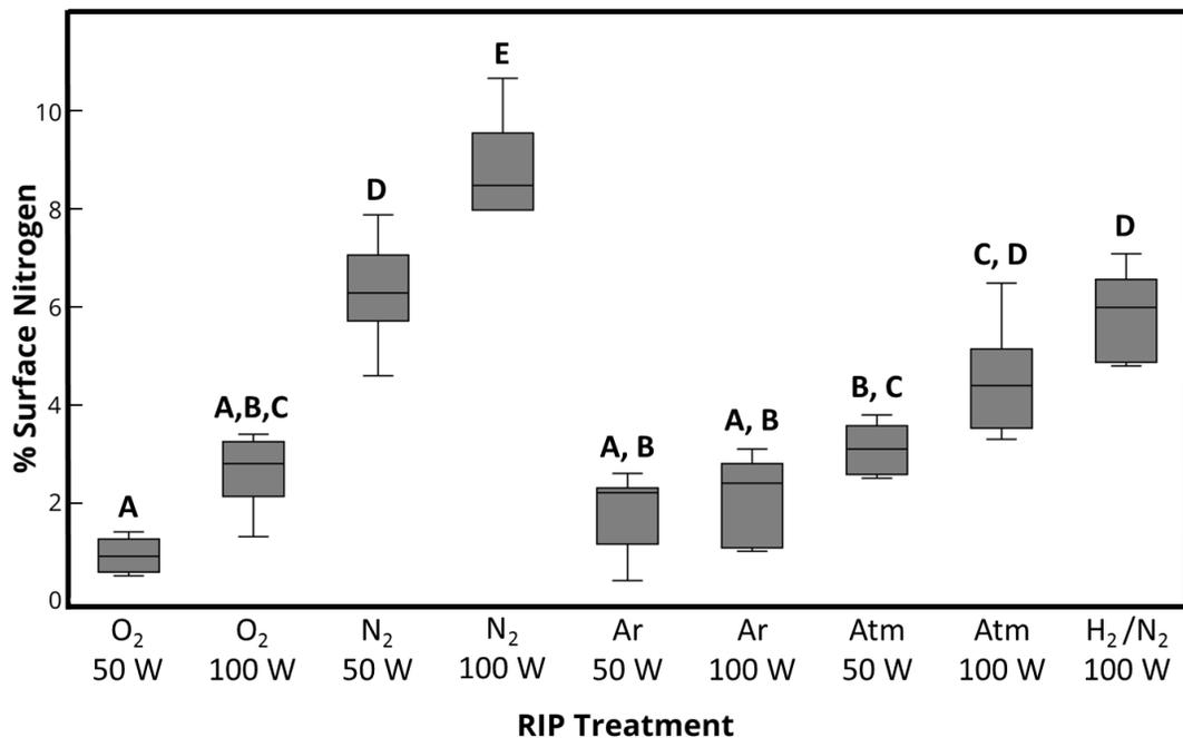
**Figure 4:** The surface nitrogen content of PVA is increased after 5 min RIP-treatment according to carrier gases and RF power. Groups which do not share a letter indicate that the null hypothesis (no statistical difference) can be rejected according to a one-way ANOVA with Tukey's post hoc ( $N = 5$ ,  $p < 0.05$ ).
