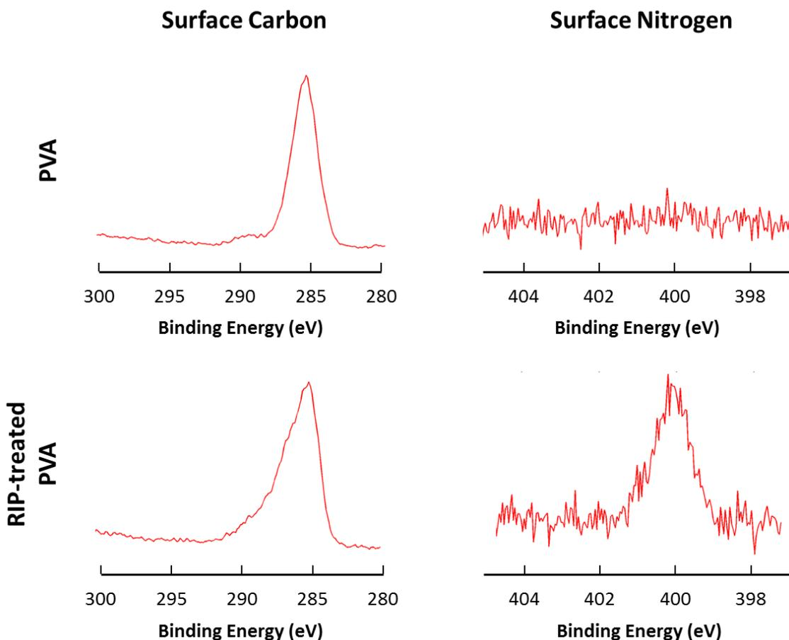
**Figure 2:** Representative high-resolution XPS spectra of surface nitrogen and carbon on native and RIP-treated PVA. Nitrogen appears on the surface of PVA after RIP treatment.
