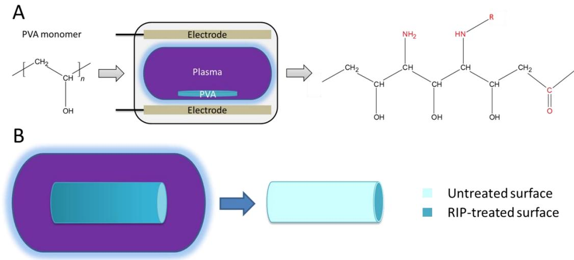
**Figure 1:** RIP treatment alters the surface chemistry of PVA. Amines and carbonyl groups, which provide binding sites for integrins, are formed on the surface (A). For *ex vivo* shunt studies PVA tubes were treated with RIP and inverted (B).
