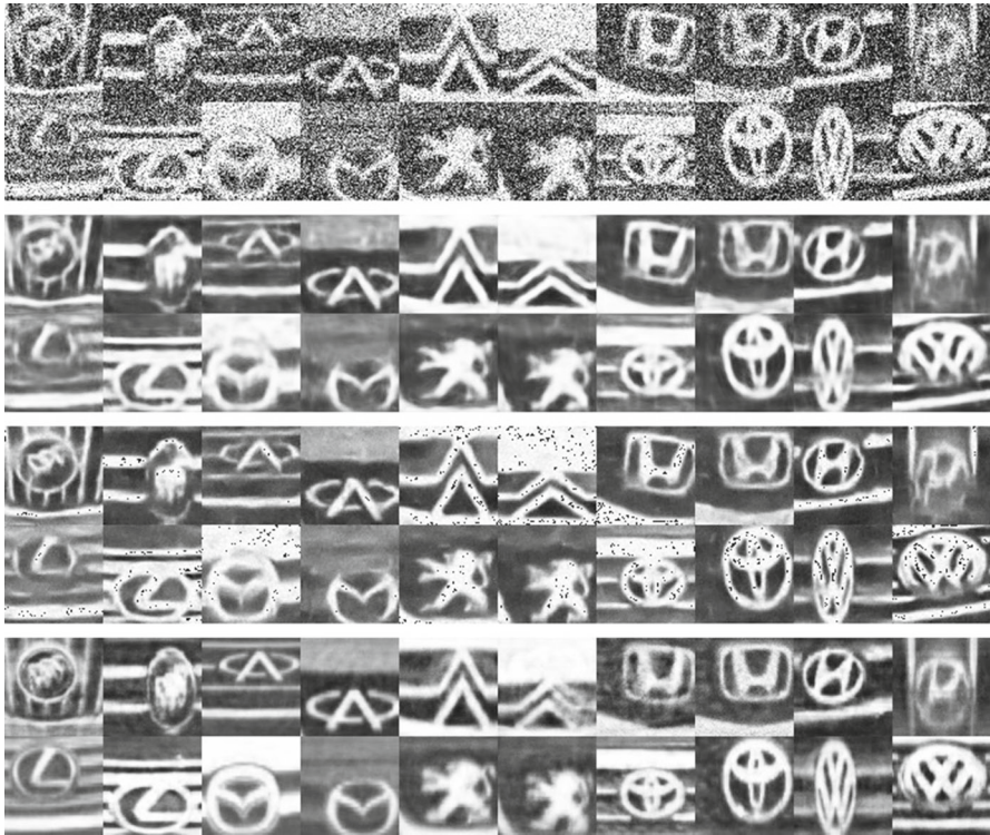
Fig. 7 First 2 rows: Noisy images. Restored images by Joint-CNN-Net, Joint-RED-Net and Joint-Cap-Net, respectively
