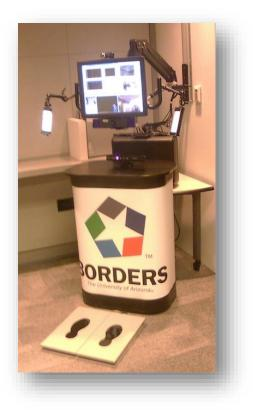
Automated Scientifically Controlled Screening Systems (ASCSS) concept. The modular design of the ASK provides flexibility in human-computer experimental designs (e.g. sitting vs. standing, customizable sensors and sensor placement, adjustable lighting). An implementation of this system is pictured in this section. Several large funded University of Arizona experiments have used and will continue to use this platform.
