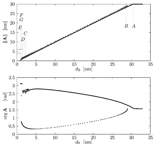
FIG. 5. Variations in magnitude  $\|\mathbf{A}\|$  and phase  $\arg \mathbf{A}$  of the complex amplitude  $\mathbf{A}$  of the frequency component of the response with frequency equal to the excitation frequency under changes in  $d_0$ . Here, a discrete fast Fourier transform has been applied to the steady-state responses found using forward-time simulation and pseudo-arclength continuation sampled 512 times per period over 20 periods of the excitation.
