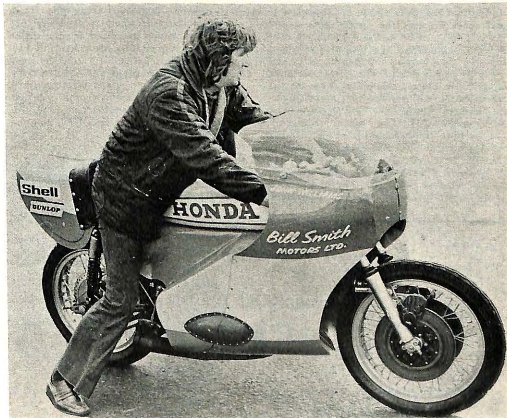
Warming up the pregnant egg: the bulge is for a Krober ignition system
