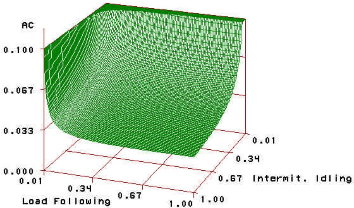
Figure 4: AC for 800 MW Gas & Oil Plants
