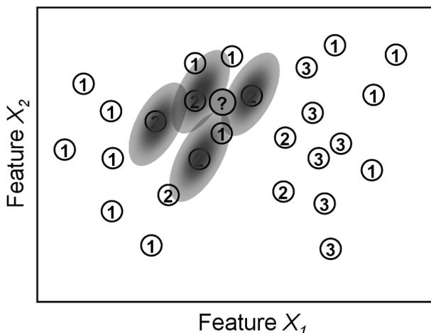
Figure 5. Parzen windows. Gaussian kernels placed over each data point are used to estimate the distribution of features in each class.
