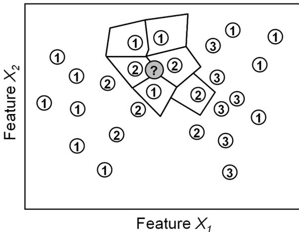
Figure 4. K-nearest neighbor. A given feature vector is assigned the class label associated with the modal class of the  $n$  samples that are the most similar to it.
