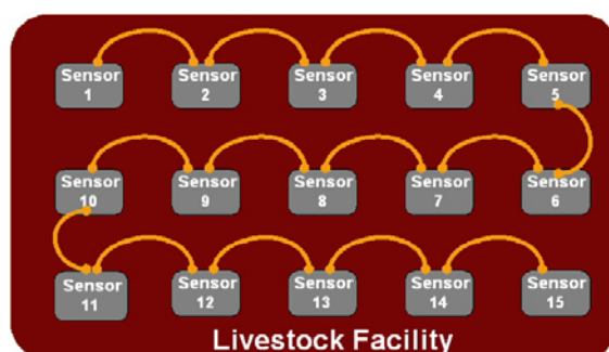
Figure 2. CAN bus installation in CAFO
