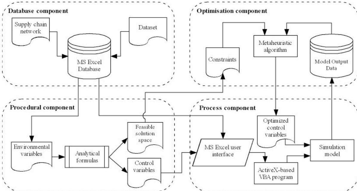
Figure 3: Architecture of Simulation-Based Environment
