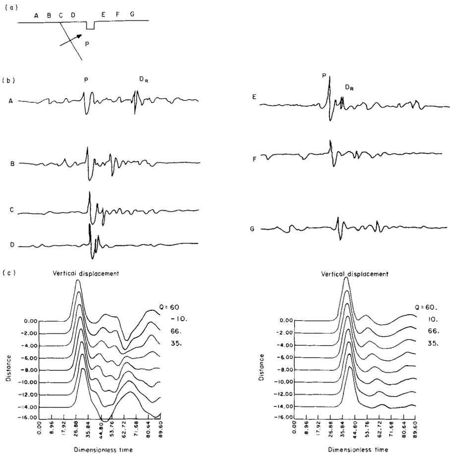
Figure 14. Experimental and numerical surface displacements for  $P$ -pulse at  $60^\circ$  and with observation points on both sides of the slot.
