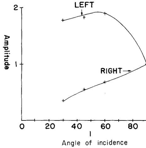
Figure 13. Experimental values of the normalized amplitude of the scattered Rayleigh pulse due to a compressional pulse of various angles of incidence at both sides of the slot.
