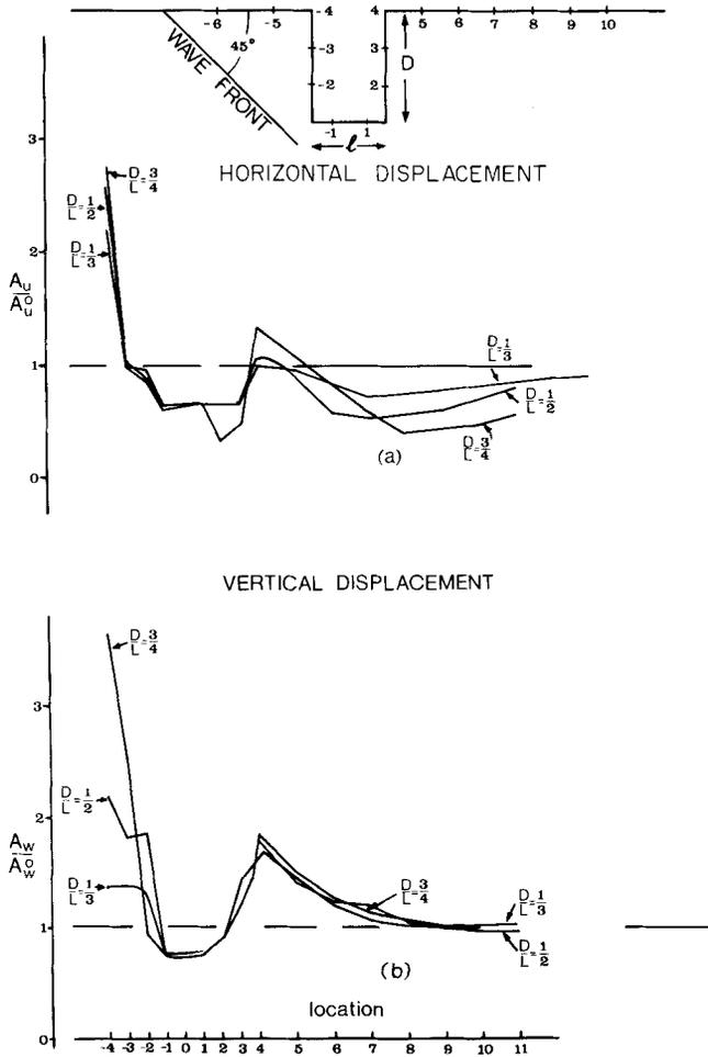
Figure 3. Relative amplitudes at 16 observation points, as defined in Fig. 2. Here the angle of incidence is  $45^\circ$  and the depth of slot varied,  $D = L/3, L/2$  and  $3L/4$ .
