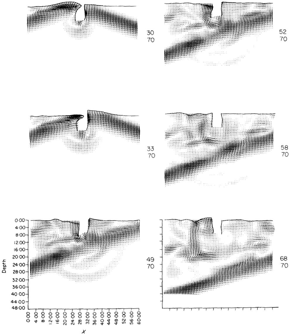
**Figure 9.** Cross-sections of the model due to a plane  $P$ -pulse at  $70^\circ$  incidence. The other details are as in Fig. 8.
