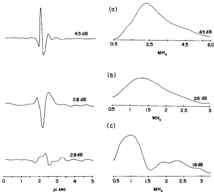
**Figure 12.** Representative results of the experiment described in Fig. 11. The vertical displacements as functions of time on the left side and the amplitude spectrum on the right. (a) The normally *P*-pulse reflected from a flat surface. (b), (c) The scattered Rayleigh pulses due to a *P*-pulse incidence at  $45^\circ$ , (b) at the front of the slot, (c) behind the slot. The depth and width of the slot are 2 and 1 mm respectively.
