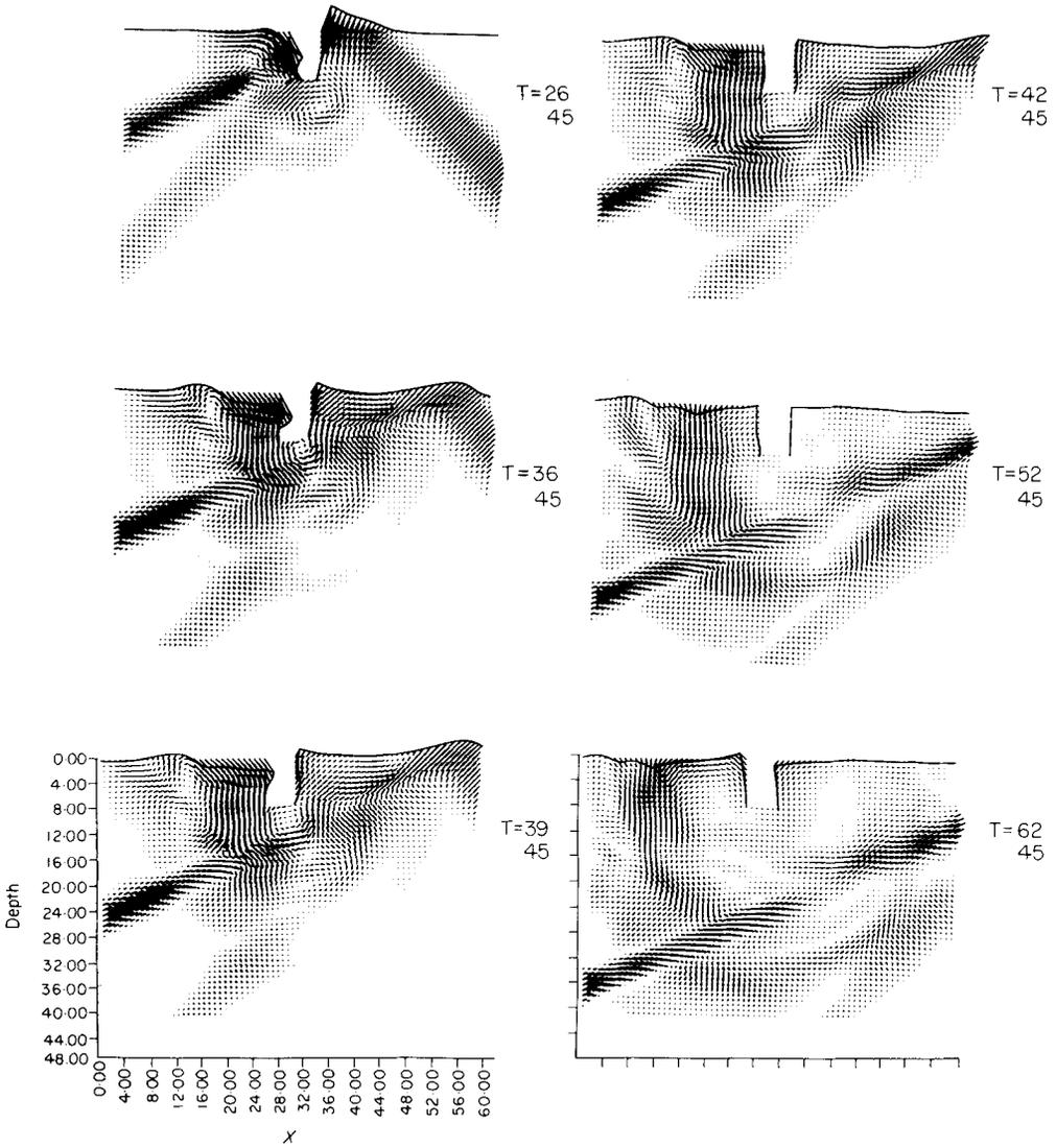
Figure 10. Cross-sections of the model due to a plane *P*-pulse at 45° incidence. The other details are as in Fig. 8.
