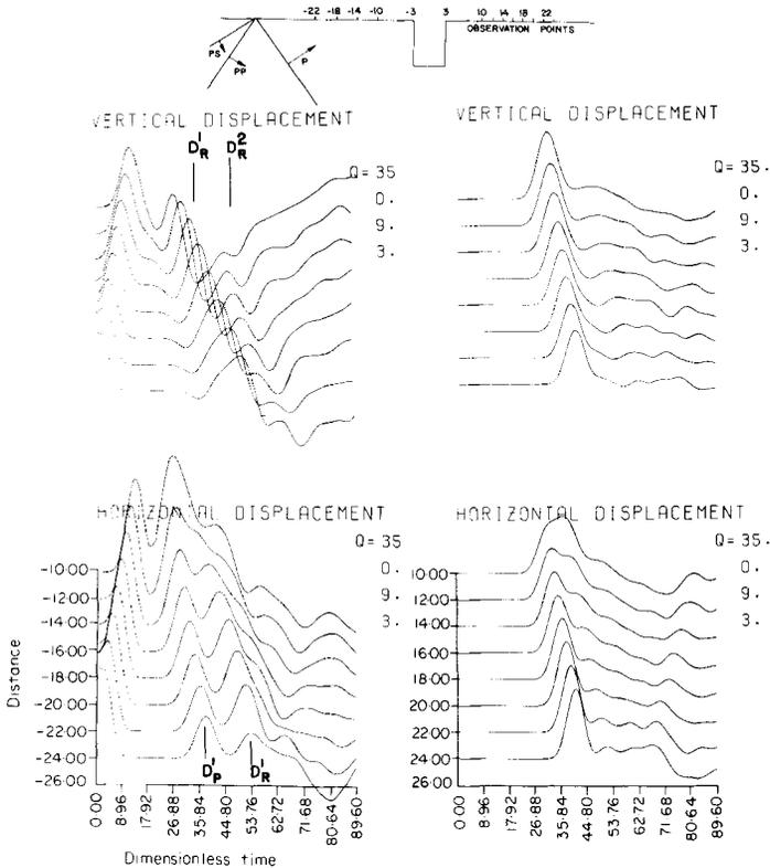
**Figure 6.** Displacements due to a plane  $P$ -pulse at  $35^\circ$  incidence as functions of  $t\alpha/h$ . The observation points are on the surface of both sides of the slot as indicated above. The dimensions of the slot are  $D=L/2$ ,  $l=L/3$ ;  $D_p^i$ ,  $D_s^i$ ,  $D_R^i$ ,  $i=1, 2$  are the scattered compressional, shear and Rayleigh waves respectively.
