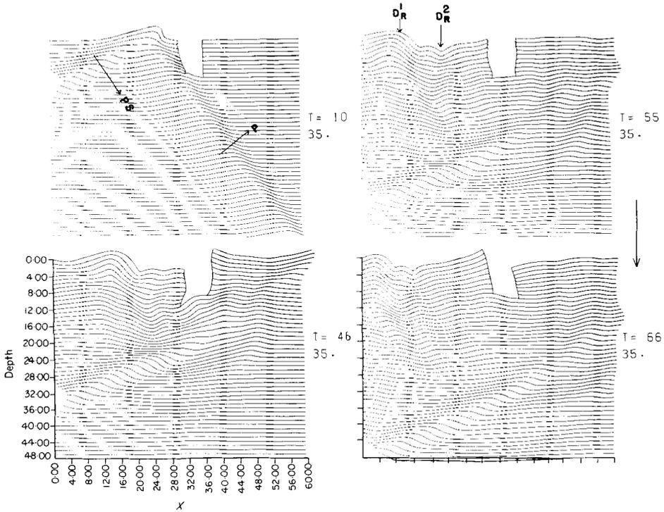
**Figure 5.** Cross-section of the model at four time levels due to a  $P$ -pulse incident at  $35^\circ$ . The times are given by the first number in each figure. The dimensions of the slot are,  $D = L/2$ ,  $l = L/3$ .  $D_R^1$  and  $D_R^2$  on the Rayleigh waves referred to in the text.
