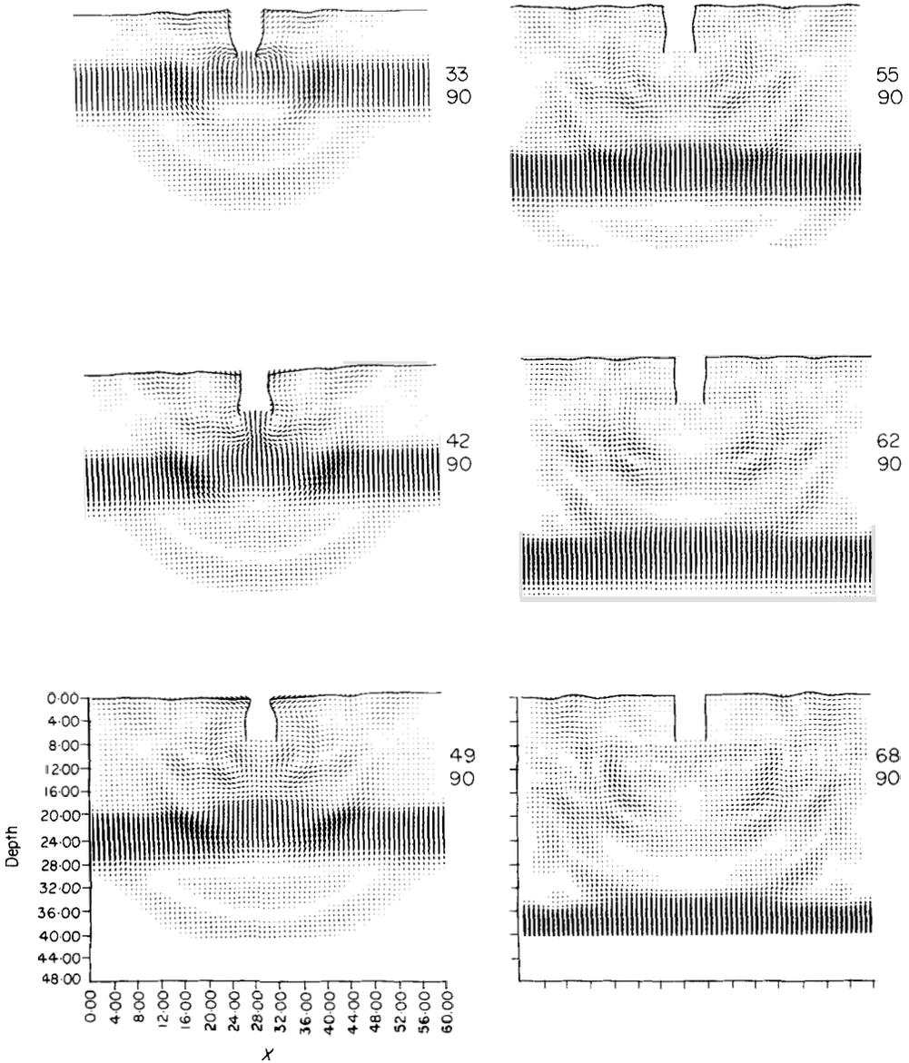
**Figure 8.** Cross-sections of the model at six consecutive time steps. The times in units of  $h/\alpha$  are indicated by the upper number in each subfigure and the lower number is the angle of incidence. The dimensions of the slot are  $D = L/2$ ,  $l = L/3$ , and the size of displacements was doubled in the graph.
