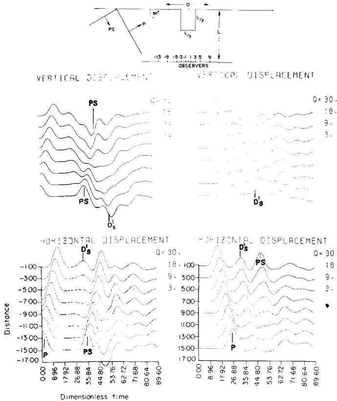
Figure 7. Displacements due to a plane  $P$ -pulse at  $30^\circ$  incidence as functions of  $t\alpha/h$ . The observation points are at a depth  $L$  below the surface, as indicated. The other details are as in Fig. 6.
