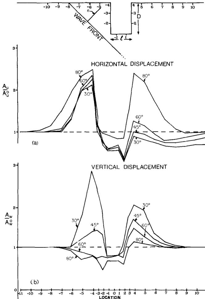
**Figure 2.**  $A_u/A_u^0$  and  $A_w/A_w^0$  at 20 observation points on the surface around a slot, as indicated above. Here  $A_u$ ,  $A_w$  are the horizontal and vertical displacement amplitudes due to  $P$ -pulses at various angles of incidence  $A_u^0$ ,  $A_w^0$  are the respective amplitudes of a  $P$ -pulse at a flat surface. Here  $l = L/3$ ,  $D = L/4$  where  $L$  is the width of the pulse.
