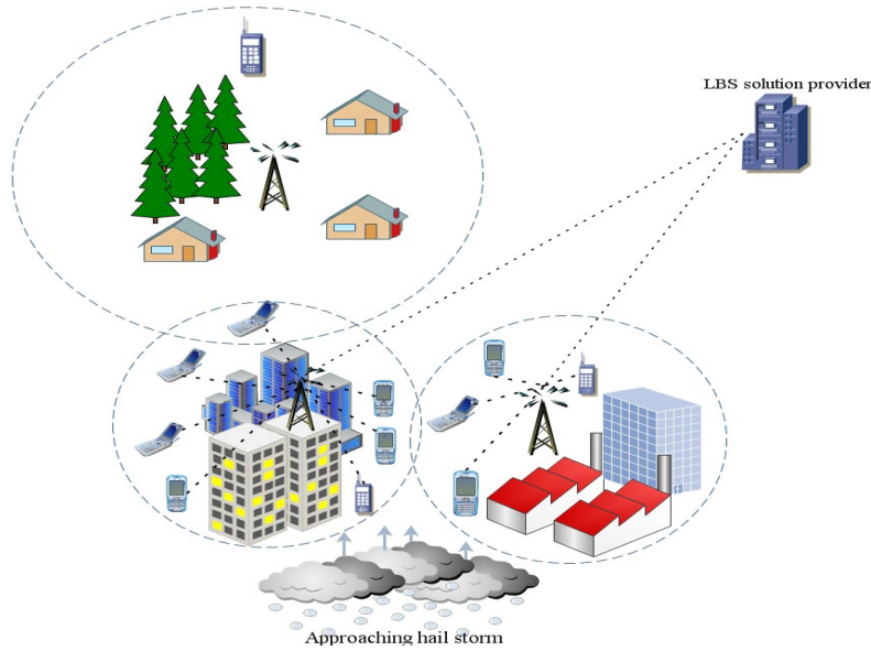
Figure 1: An example of delivering a blanket information message service about an impending hazard based upon the geo-location of the active handset
