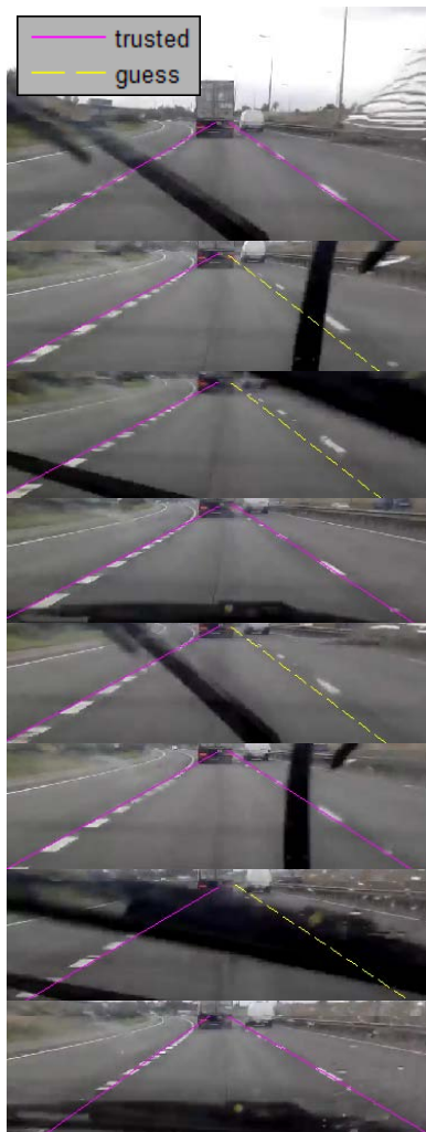
Figure 8: Successful lane boundary detection while raining.
