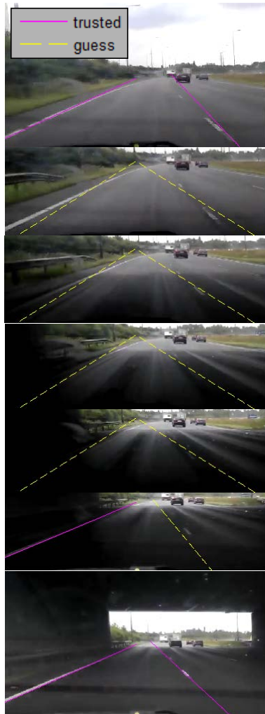
Figure 12: Changing light conditions entering an underpass and the resulting loss of lane boundary detection.
