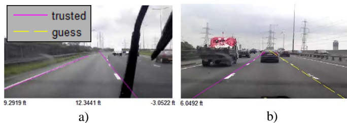
Figure 6: Road images where a) both detected lane boundaries are trusted and b) where one boundary is trusted and the other is approximated.
