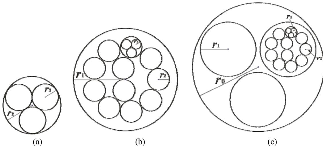
Fig. 2 diagrams of three hierarchic levels of wool fibre
