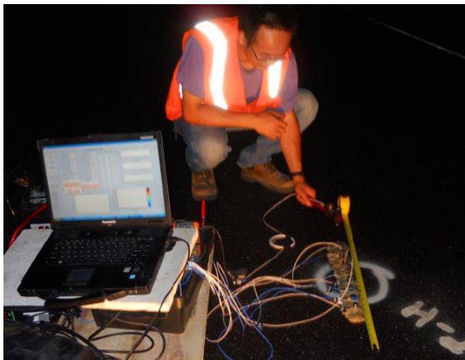
Figure 1. Surface wave testing on US 6
