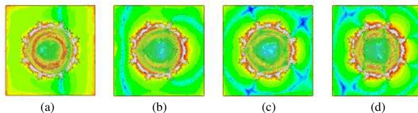
Figure 4: The simulated surface current distribution on the modelled antenna with circular stub of 17 mm radius and embedded CCSR with inner radius of 5 mm at: (a)  $f_1=1.54$  GHz, (b)  $f_2=2.40$  GHz, (c)  $f_3=4.00$  GHz, and (d)  $f_4=5.20$  GHz.
