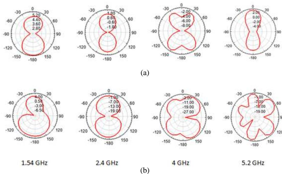
Figure 3: The simulated far field radiation patterns of the modelled antenna with circular stub of 17 mm radius and embedded CCSR with inner radius of 5 mm at the four resonant bands. (a) The  $E$ -plane, and (b) the  $H$ -plane.
