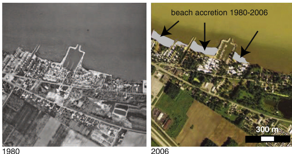
Fig. 11. Comparison of aerial photographs from May 6, 1980 and July 26, 2006, showing sand accumulation updrift of the Portage River delta. Incorporation of the digitized images into a GIS database permits calculating the areal extent of the beaches, and core data was used to calculate sand volumes. Scale shown in lower right corner. See text for discussion.
