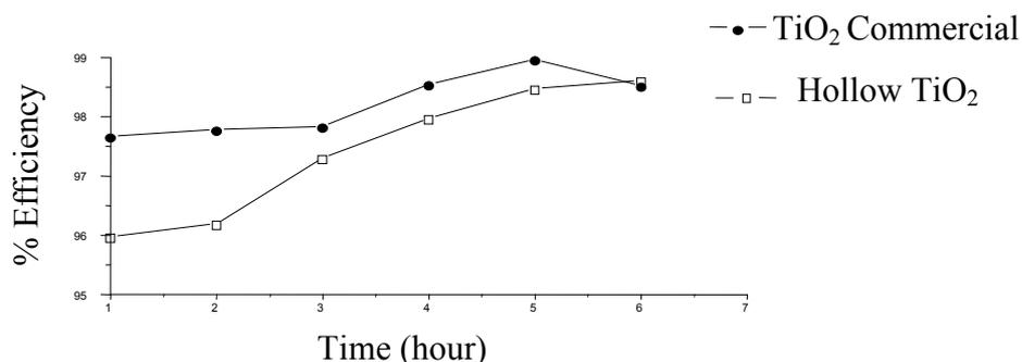
Fig. 6 Plots of the efficiency of hollow TiO<sub>2</sub> and commercial TiO<sub>2</sub> against irradiation time of UV.
