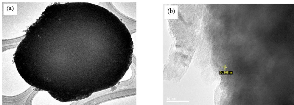
Fig. 2 (a) TEM image of hollow anatase TiO<sub>2</sub> spheres prepared by template method and (b) HRTEM image of the selected particle.
