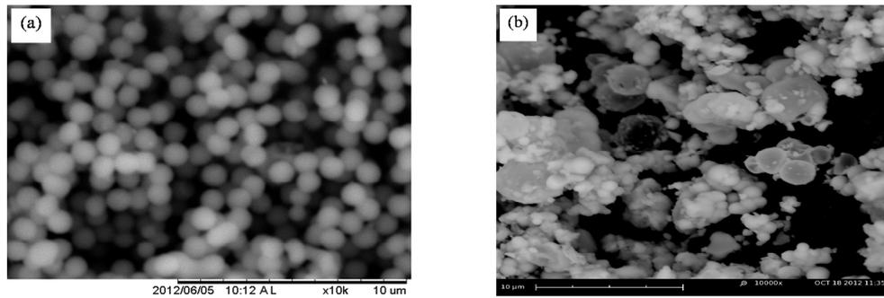
Fig. 1 SEM image of (a) carbon spheres formed by heating at 160 °C for 5 h and FESEM image of (b) hollow TiO<sub>2</sub> spheres
