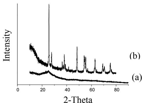
Fig. 4 XRD patterns of (a) carbon and (b) hollow anatase TiO<sub>2</sub> spheres.
