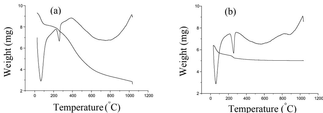
Fig. 5 TG–DTA curves of (a) carbon spheres and (b) hollow TiO<sub>2</sub> spheres.
