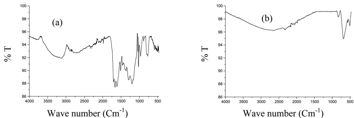
Fig. 3 FTIR spectra of (a) carbon spheres prepared by hydrothermal method and (b) hollow TiO<sub>2</sub> spheres.
