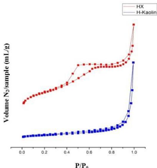
Fig. 6 The Isotherm N<sub>2</sub> Adsorption-Desorption of HX and H-kaolin.
