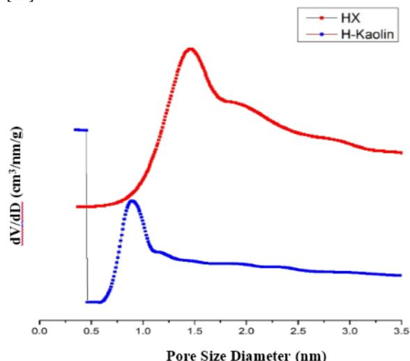
Fig. 8 The micropore distribution of as-synthesized HX from the SF method
