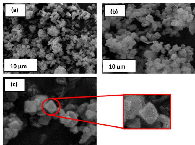
Fig. 5 The SEM micrograph of synthesized NaX.
