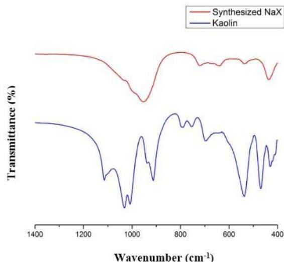
Fig. 4 The Spectra FTIR of synthesized NaX and kaolin.
