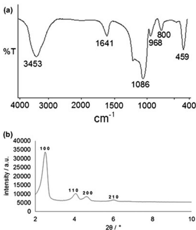
**FIGURE 2** FTIR (a) and XRD (b) results of synthesized MCM-41
