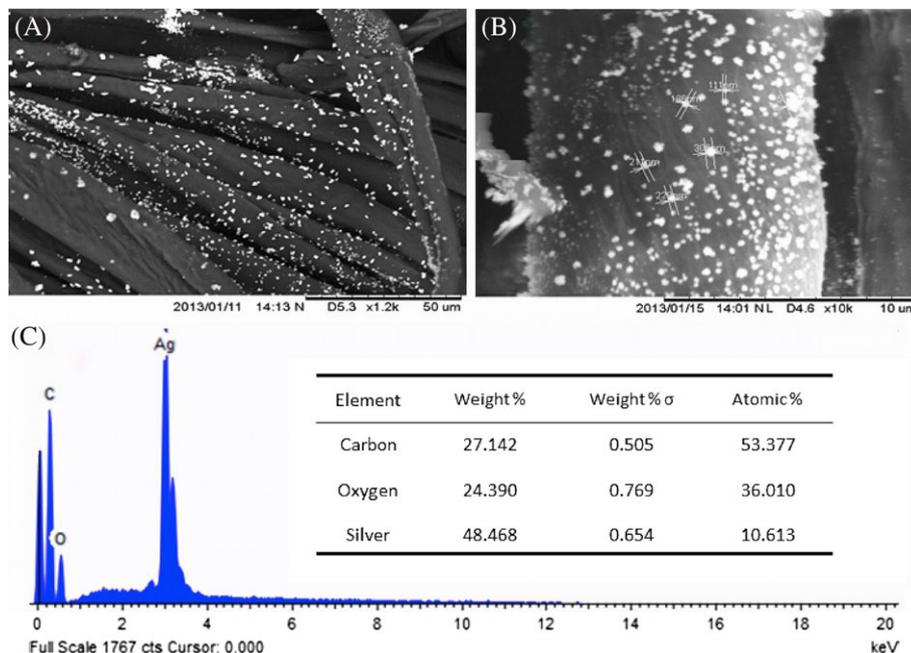
Fig. 2. SEM images of Ag-NP/cotton nanocomposite (sample C (0.05 M)) with different magnifications (a)  $\times 1200$  and (b)  $\times 10\,000$ . (c) EDS image from Ag-NP/cotton nanocomposite.
