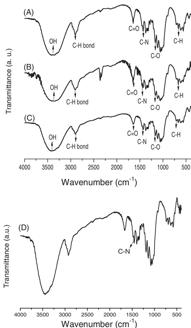
Fig. 1. FTIR spectra of sample A (0.005 M), B (0.01 M), C (0.05 M), and D (cotton).
