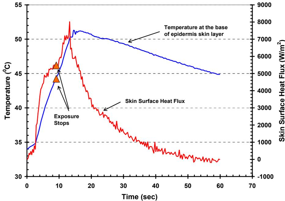
FIG. 8—Calculated skin surface heat flux and temperature change at the base of epidermis behind the composite exposed to  $2.0 \text{ cal/cm}^2 \cdot \text{s}$  ( $83.7 \text{ kW/m}^2$ ) for 10 s.
