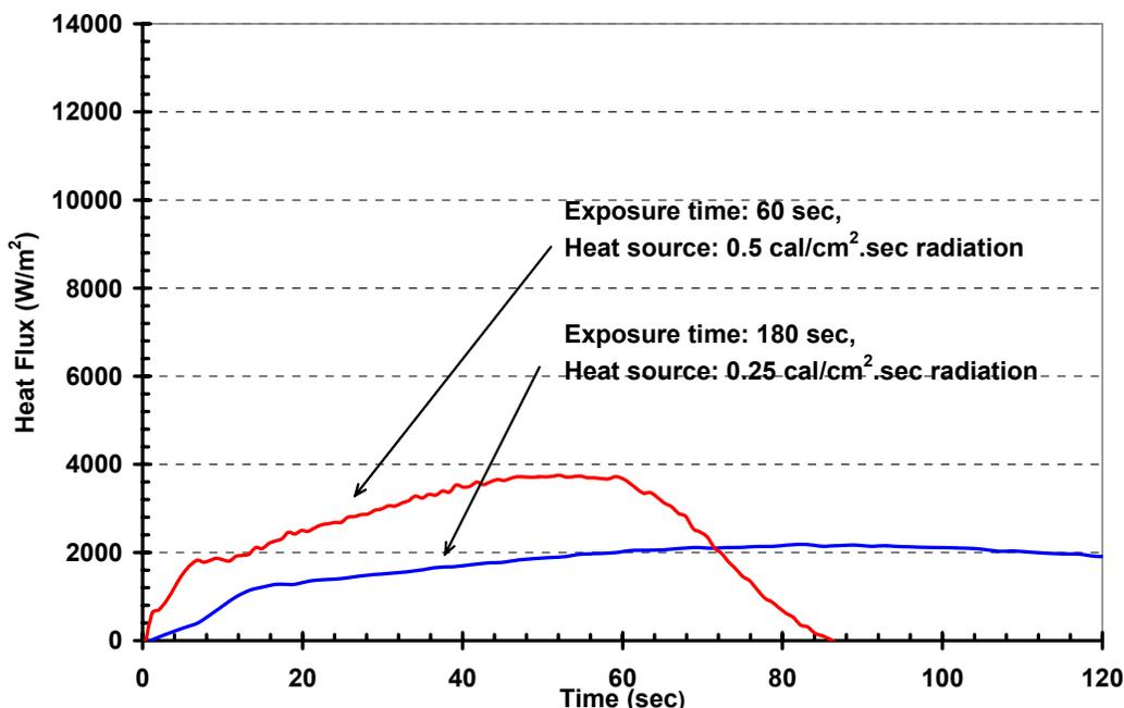
FIG. 5—Heat flux profiles under firefighter turnout systems exposed to low radiation thermal conditions.
