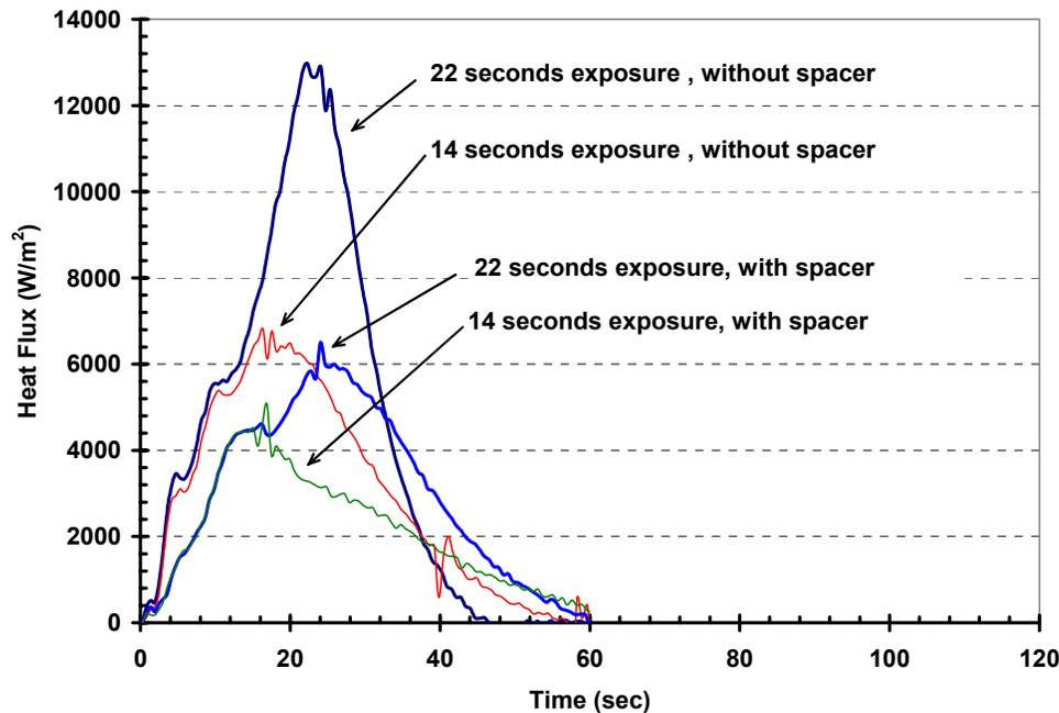
FIG. 6—Heat flux profiles behind ensembles exposed to  $2.0 \text{ cal/cm}^2 \cdot \text{s}$  in dry condition.
