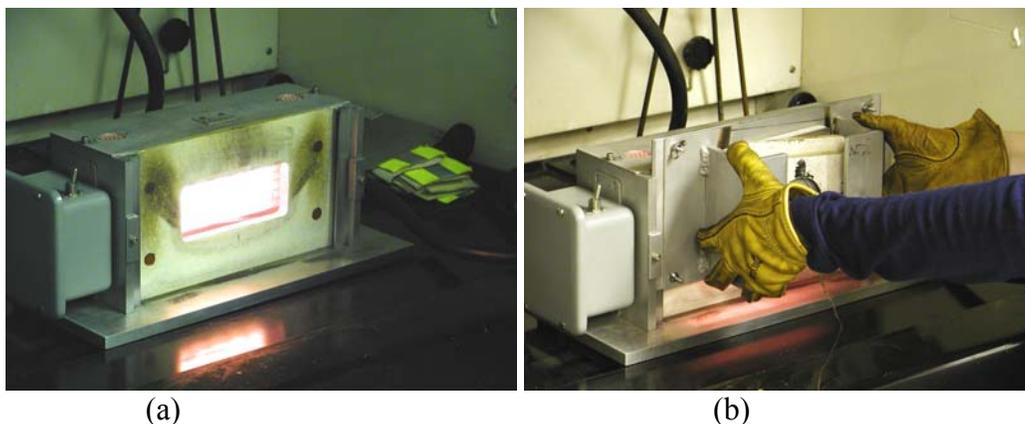
FIG. 2—RPP tester: (a) Heat source, (b) Sample mounting and Copper Calorimeter.
