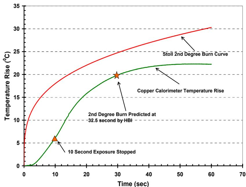
FIG. 7—*Measured temperature rise behind the composite exposed to 2.0 cal/cm<sup>2</sup>·s for 10 s in wet condition.*
