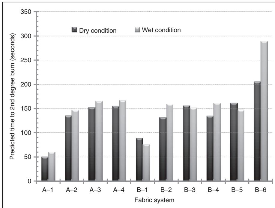
**Figure 8.** Comparison of predicted time to second degree skin burn in standard and wet conditions when exposed to 7.5 kW/m<sup>2</sup>.
