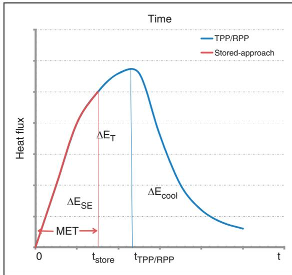
**Figure 5.** Schematic of heat flux profiles for TPP/RPP approach and stored-energy approach.
