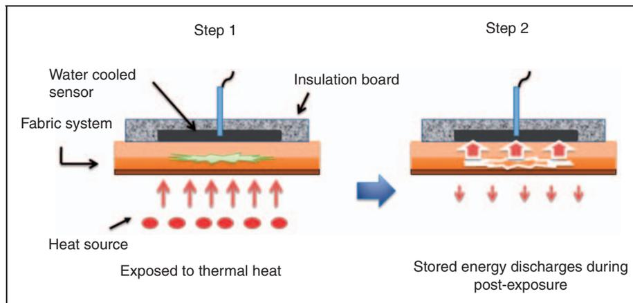
Figure 4. Stored-energy test schematic procedure for data collection.
