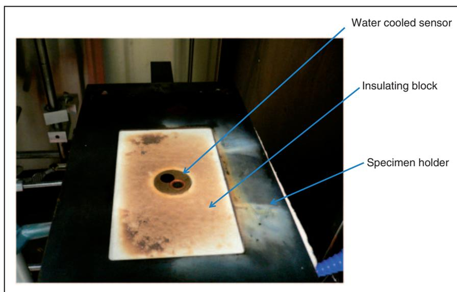
**Figure 1.** Specimen holder and water cooled sensor used in the apparatus.
