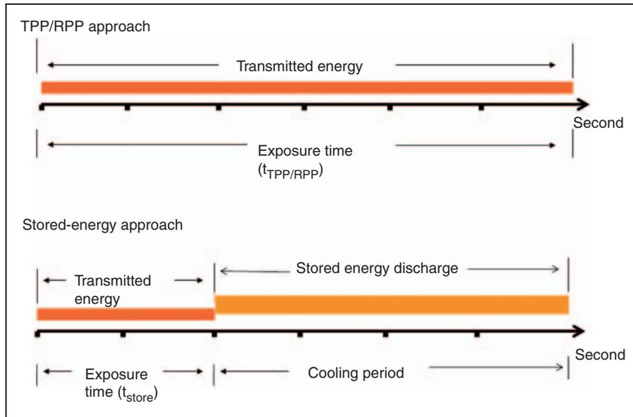
Figure 3. Comparison of the TPP/RPP and stored energy approach.
