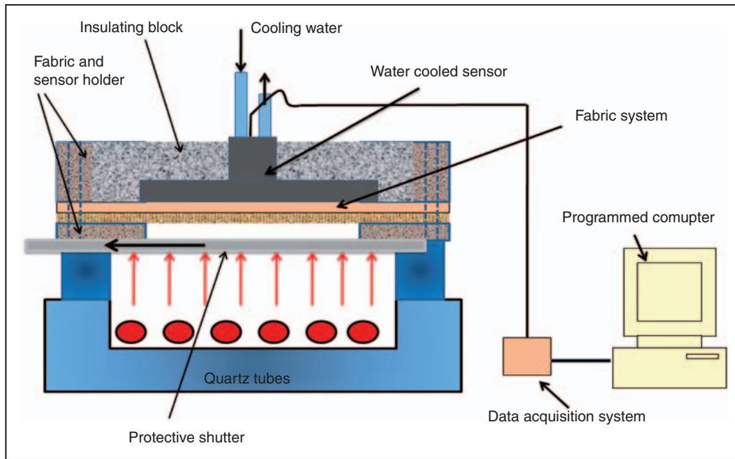
**Figure 2.** Schematic diagram of apparatus used to measure thermal protective performance.
