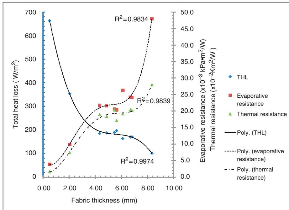
**Figure 10.** The effect of fabric thickness on thermal resistance, evaporative resistance and total heat loss. Poly. represents a polynomial regression for selected data series.
