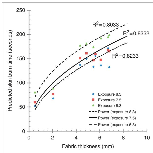
**Figure 7.** Effect of fabric system thickness on predicted skin burn time in wet condition. Power represents a power regression for selected data series.
