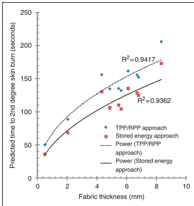
**Figure 9.** Comparison of predicted burn time from TPP/RPP to MET for stored energy at exposure of  $7.5 \text{ kW/m}^2$ . Power represents power regression for selected data series.
