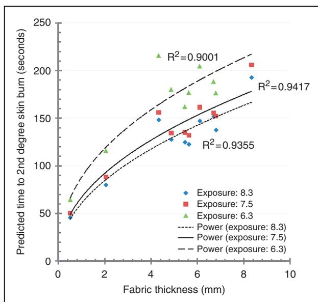
**Figure 6.** Effect of fabric system thickness on predicted skin burn time under different exposure level. Power represents a power regression for selected data series.
