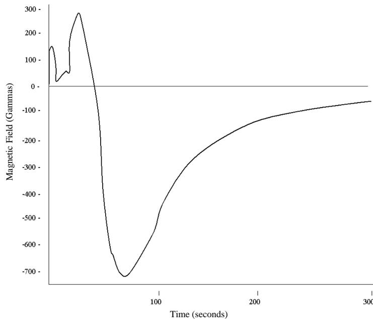
**Figure 4. Magnetometer data from the Starfish nuclear test
