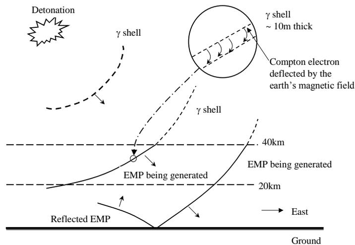
Figure 1. Mechanism of gamma-induced EMP from a high-altitude burst
