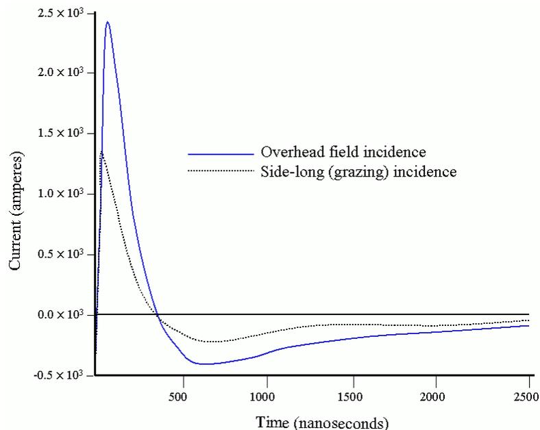
Figure 5. EMP-induced current on overhead power line
