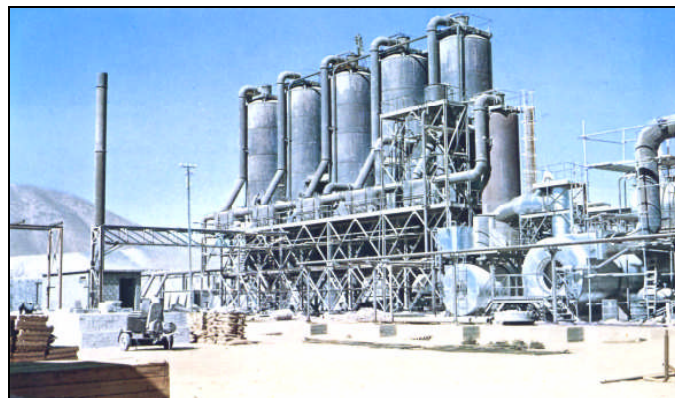
Figure 75. Sulfur dioxide towers for precipitating \text{Cu}_2\text{Cl}_2 .
