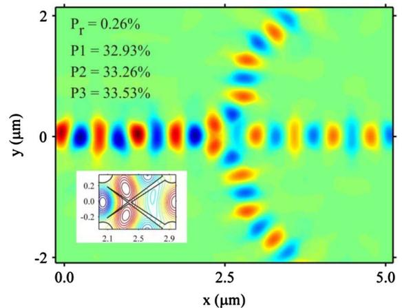
Fig. 5. Steady-state magnetic field ( $H_z$ ) distribution at  $L = 2.3\Lambda$ ,  $r1 = 0.25r$  and  $\theta = \pm 35^\circ$  at 1550 nm wavelength. The inset shows the contour plot at the junction area.
