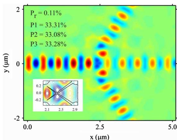
Fig. 10. Steady-state magnetic field ( $H_z$ ) distribution for  $L = 2.3\lambda$ ,  $r1 = 0.25r$  and  $\theta = \pm 35^\circ$  at 1388 nm wavelength. The inset shows the contour plot at the junction area.
