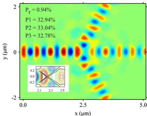
Fig. 11. Steady-state magnetic field ( $H_z$ ) distribution for  $L = 2.3\lambda$ ,  $r1 = 0.25r$  and  $\theta = \pm 35^\circ$  at 1470 nm wavelength. The inset shows the contour plot at the junction area.
