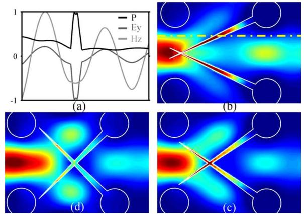
Fig. 8. Field distribution for different bending angles. (a) Field amplitude corresponding to the dash-dot line (yellow) in (b), where P is the power,  $E_y$  is the y-component of the electric field vector and  $H_z$  is z-component of the magnetic field vector. Power distribution (b) at bending angle of  $25^\circ$ , (c) at bending angle of  $35^\circ$ , and (d) at bending angle of  $45^\circ$ .
