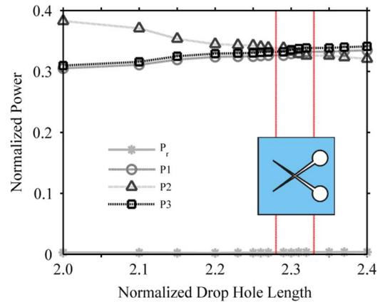
Fig. 4. Normalized output transmission and reflection power versus drop hole length  $L$  normalized with respect to lattice constant  $\Lambda$  at  $r1 = 0.25r$  and  $\theta = \pm 35^\circ$ . The interval between the vertical red lines indicates the optimum operation region. The optimum region is calculated based on the computation accuracy of the simulation. The inset shows the layout of the drop holes at  $L = 2.3\Lambda$ .
