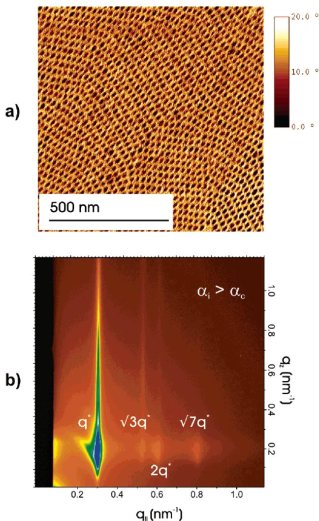
**Figure 7.** (a) Tapping mode SFM phase image. (b) GISAXS pattern at an incident angle of  $0.12^\circ$ ,  $\lambda = 0.1042$  nm, of  $\text{CEC}_{50,24,10}$  annealed at  $220^\circ\text{C}$  for 3 days.
