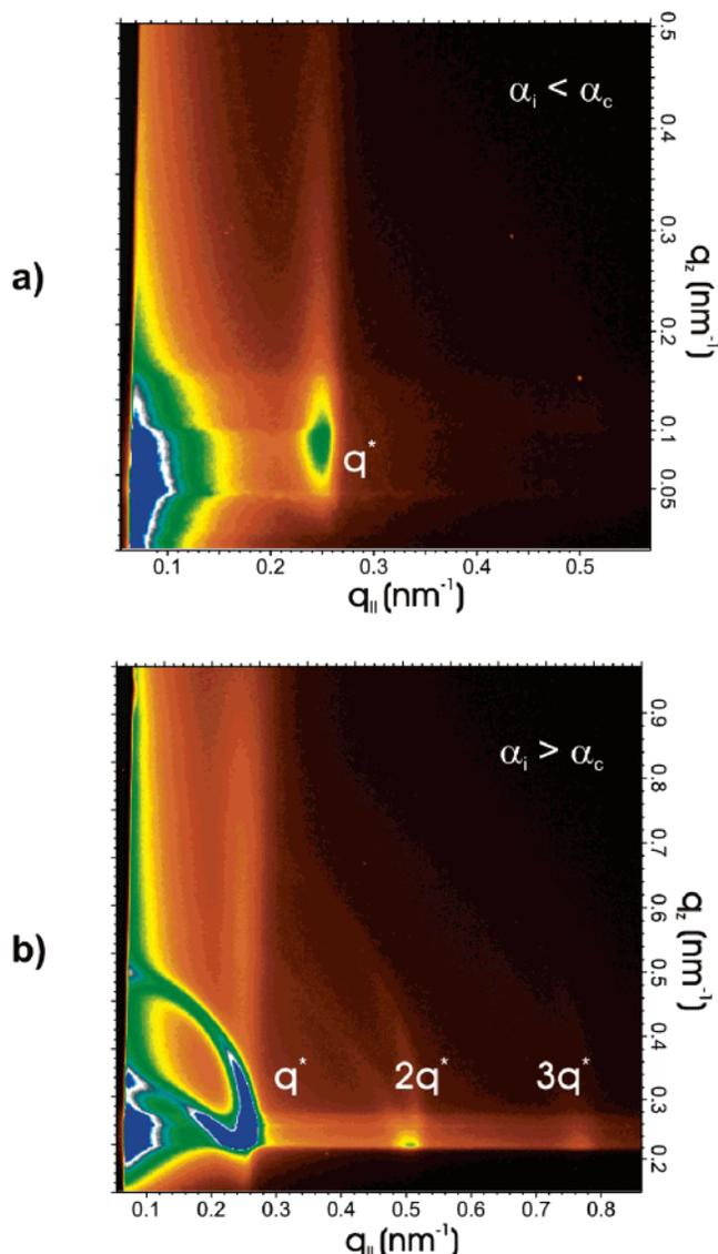
**Figure 5.** GISAXS pattern ( $\lambda = 0.1675 \text{ nm}$ ) at an incident angle of (a)  $0.06^\circ$  and (b)  $0.21^\circ$  of  $\text{CEC}_{45.48.10}$  annealed at  $220^\circ \text{C}$  for 3 days.
