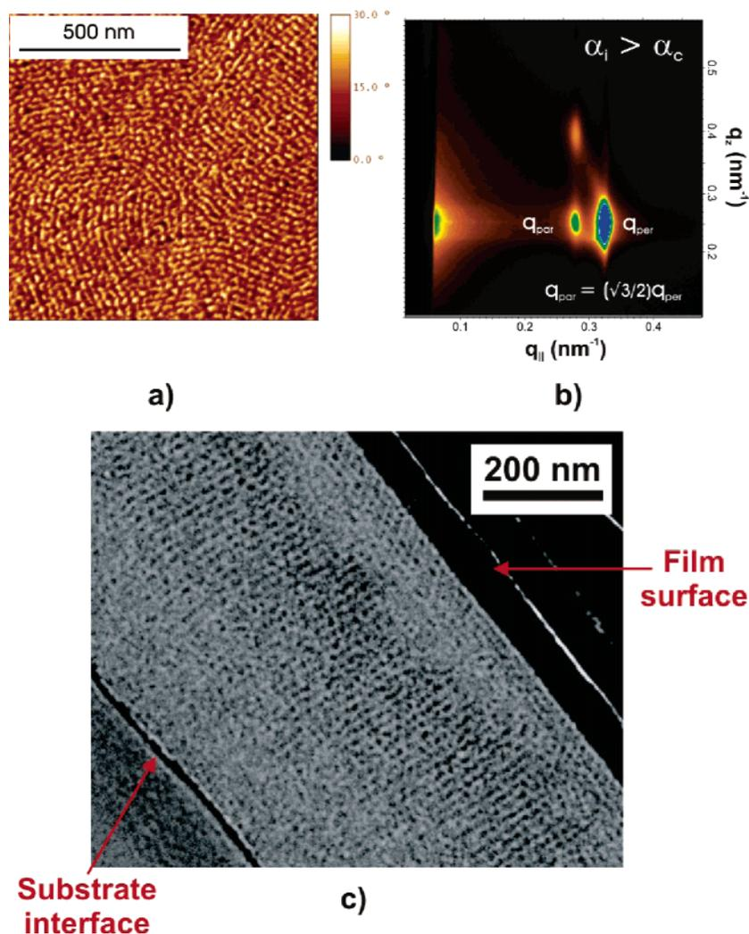
**Figure 8.** (a) Tapping mode SFM phase image. (b) GISAXS pattern at an incident angle of  $0.21^\circ$ ,  $\lambda = 0.1675$  nm. (c) Cross-sectional TEM image of CEC<sub>60.24.40</sub> annealed at  $220^\circ\text{C}$  for 4 days. The E block contains about 1 ethyl branch per 8 backbone carbons due to the 40% 1,2 monomer addition in the PB precursor.
