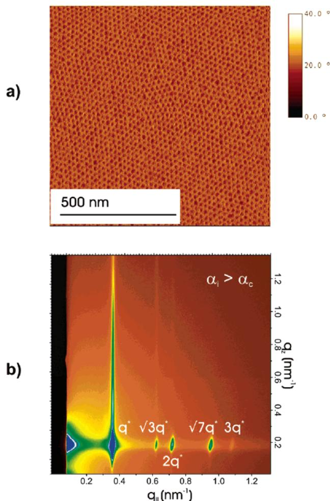
**Figure 6.** (a) Tapping mode SFM phase image. (b) GISAXS pattern at an incident angle of  $0.12^\circ$ ,  $\lambda = 0.1042 \text{ nm}$ , of  $\text{CEC}_{40.25.10}$  annealed at  $220^\circ \text{C}$  for 3 days.
