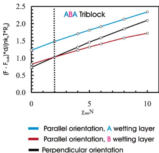
**Figure 10.** Self-consistent-field theory calculations for 37/25/38 ABA triblock copolymer showing the excess free energy for different orientations as a function of  $\chi_{AW}N$ . The equilibrium morphology is cylindrical. The dotted line indicates the value of  $\chi_{AW}N$  at which the parallel orientation, with a B wetting layer, becomes energetically more favorable than the perpendicular orientation.
