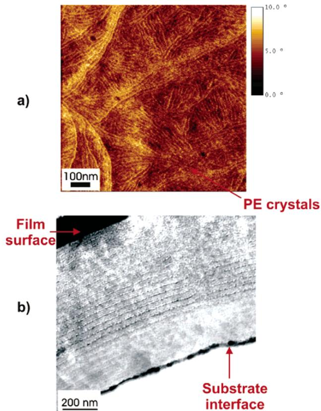
**Figure 3.** CE<sub>22,48,10</sub> annealed at 220 °C for 3 days: (a) Tapping mode SFM phase image; (b) cross-sectional TEM image.
