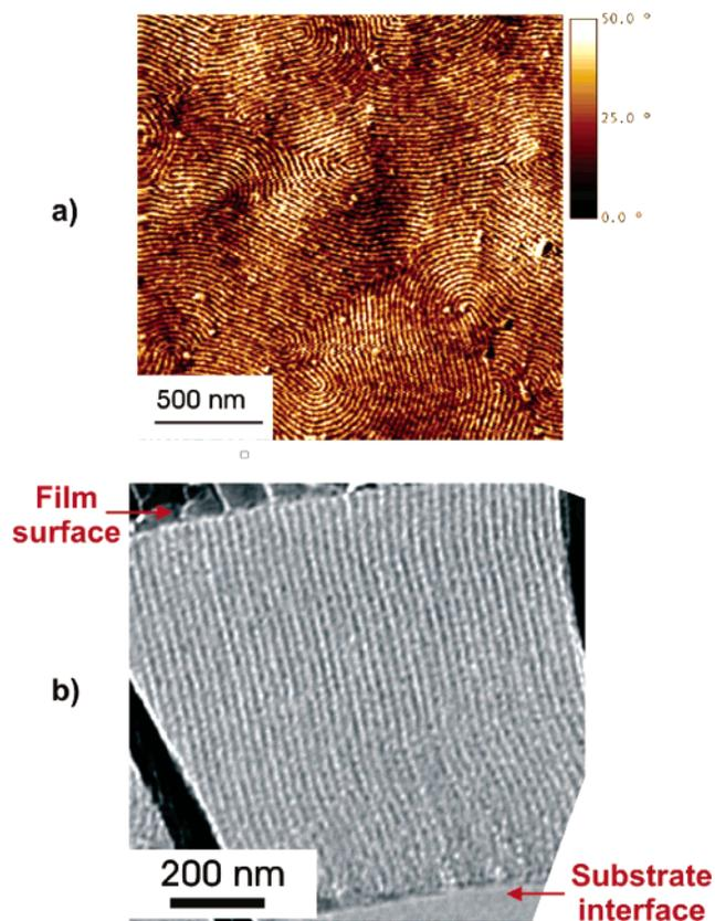
**Figure 4.** CEC<sub>45,48,10</sub> annealed at 220 °C for 3 days: (a) Tapping mode SFM phase image; (b) cross-sectional TEM image.
