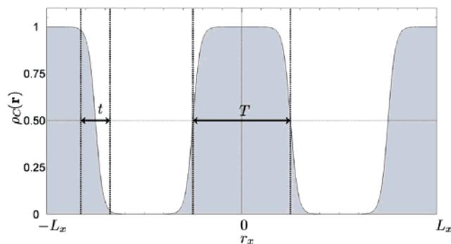
**Figure 2.** Film geometry corresponding to eq 4 showing the depth profile of the interfacial density field for two unit cells (two thin films). Here  $t = 0.15L_x$  and  $T = 0.5L_x$ . Incompressibility renders the shaded regions inaccessible to the block copolymer. Surface interactions are manifested through the overlap region of width  $t$  where  $0 \lesssim \rho_w(\mathbf{r}) \lesssim 1$ .
