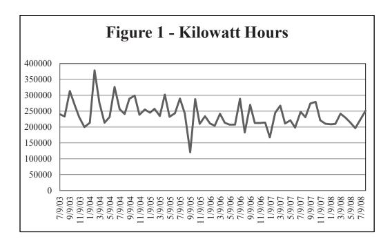
Curiously, there appears to be no seasonality in kilowatt hours. Standard tests for seasonality (F-test, Kruskall-Wallis) reveal that there is none. Given the assumption of no trend and the lack of seasonality, the mean of the kilowatt hour variable (239,173) is selected to represent the typical value that occurs over the life of the proposed project.
