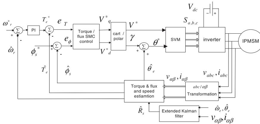
Fig. 2. Block diagram of the sensorless torque/flux SMC-SVM scheme.
