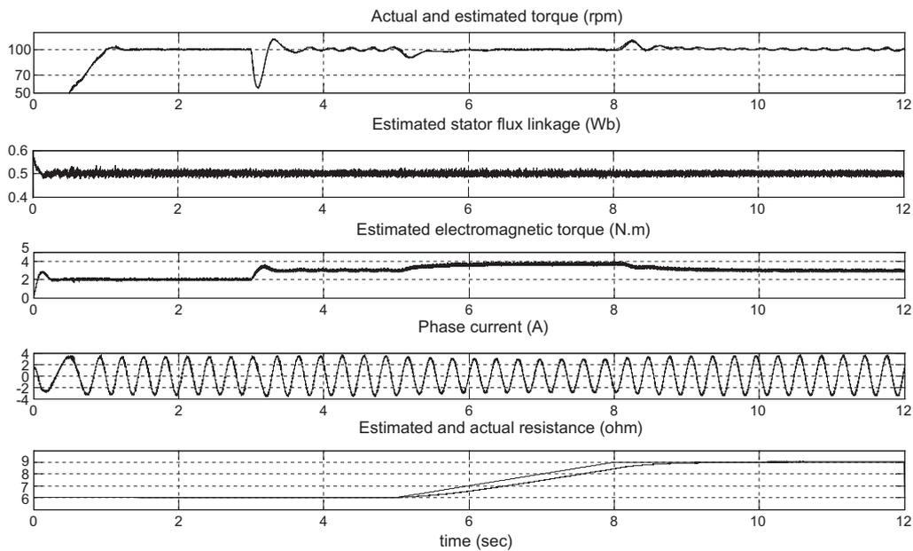
**Fig. 3.** Simulation waveforms of the sensorless torque/flux SMC scheme (low speed operation).
