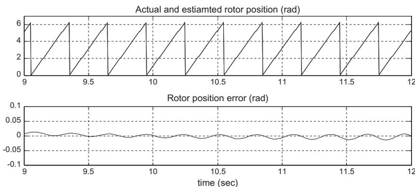
**Fig. 4.** Actual and estimated rotor position waveforms and the position angle error (low speed operation).
