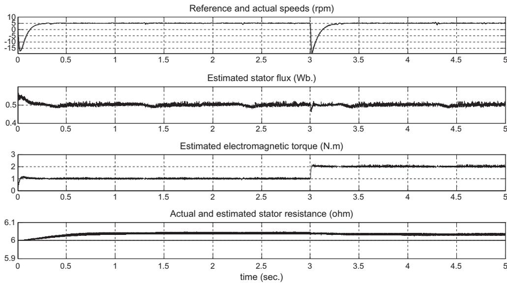
Fig. 5. Simulation waveforms of the sensorless torque/flux SMC scheme (very low speed operation).
