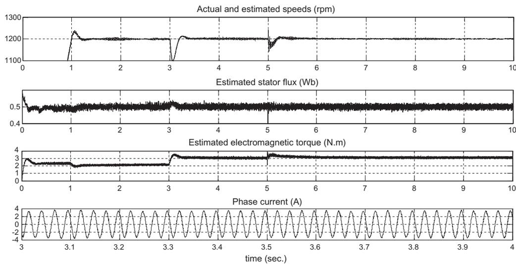
Fig. 7. Simulation waveforms of the sensorless torque/flux SMC scheme (high speed operation).
