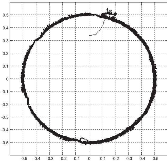
Fig. 6. Locus of the stator flux of the torque/flux SMC in the stationary frame (very low speed).
