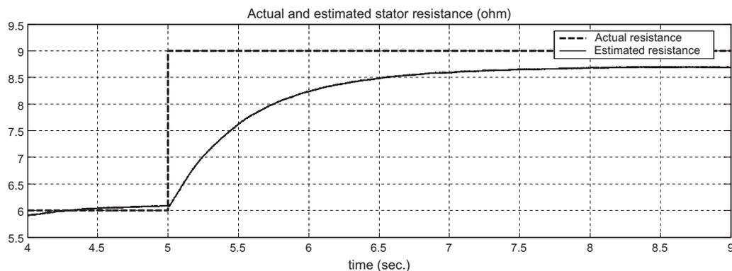
Fig. 8. Actual and estimated stator resistances waveforms (high speed operation).
