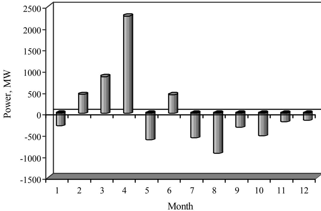
Fig. 4-7 The Total Power Surplus and Deficit Power for each Month for T600-48 Wind Turbine Type for Zafarâna site, Egypt.
