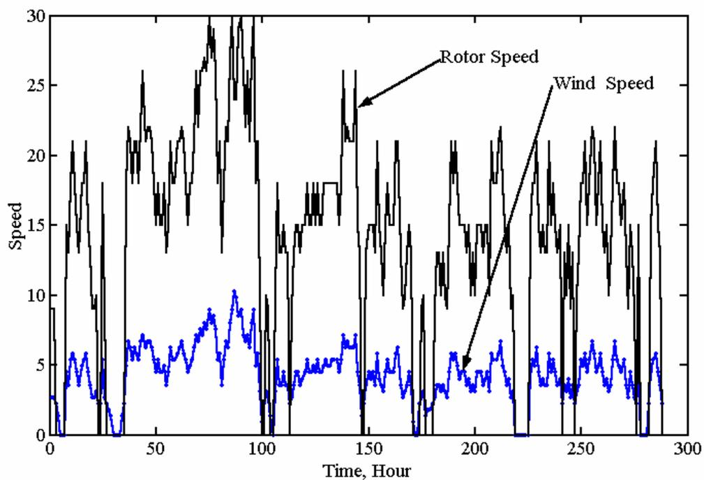
Fig. 4-9 Variations of Wind Speed and Rotor Speed with time
