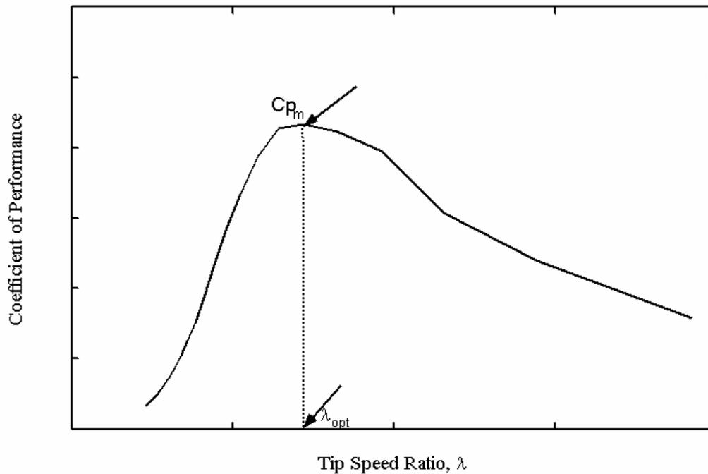
Fig. 4-1 Coefficient of Performance Versus tip speed ratio
