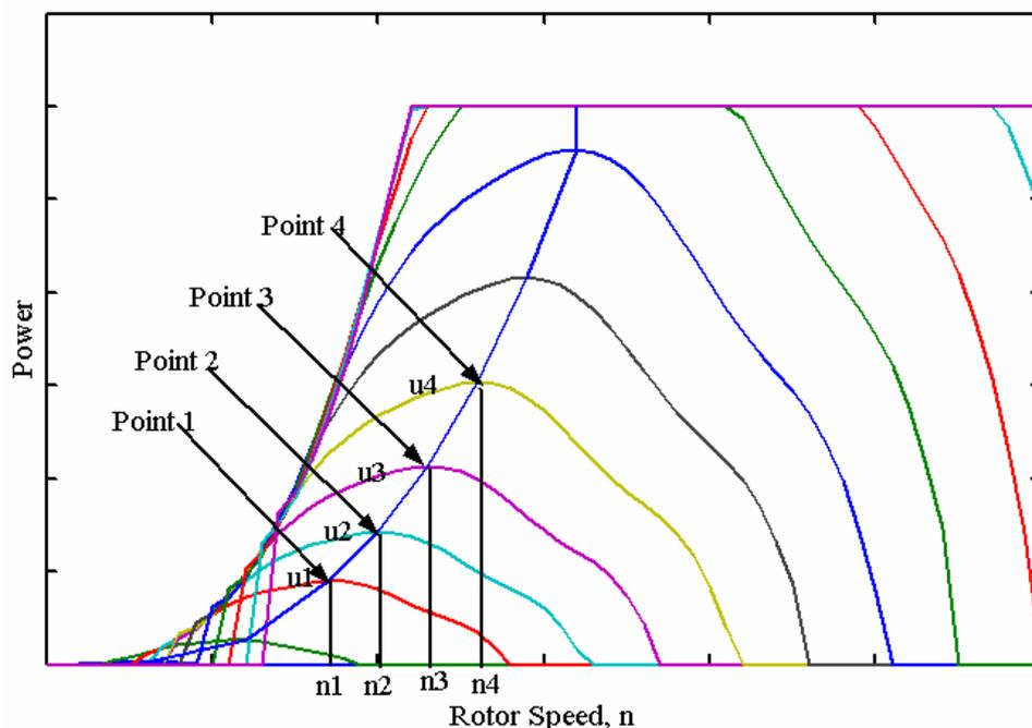
Fig. 4-2 Shaft Power Output Versus Generator Speed
