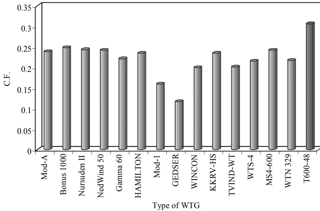
Fig. 4-5 The Capacity Factor of the Selected WTG's for Zafarâna site, Egypt.
