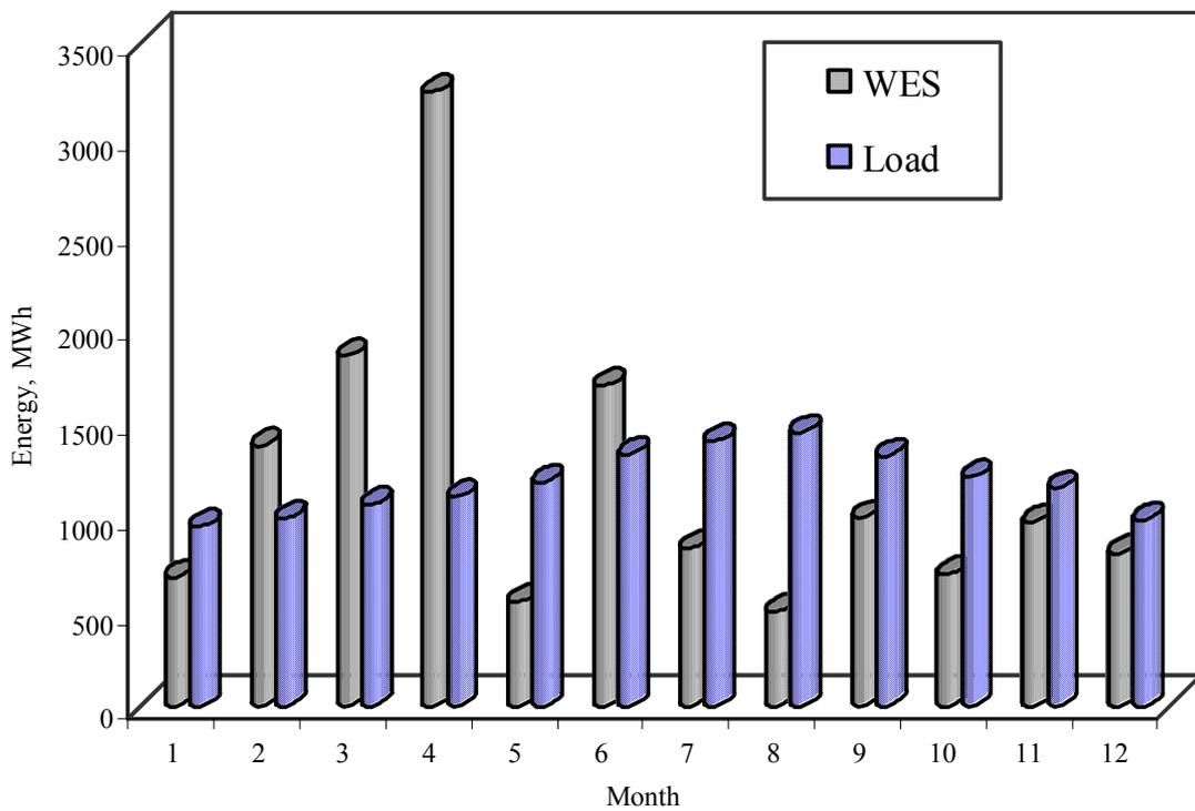
Fig. 4-8 The Total Energy Generated and Energy Demand for each Month for T600-48 Wind Turbine Type.
